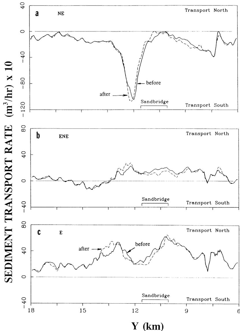
Figure 11. Comparison of longshore sediment transport rates before (solid line) and after (dashed line) the modeled dredging at Sandbridge Shoal for the most severe sea ( $H = 6.2$  m,  $T = 20$  sec) coming from (a) NE; (b) ENE; and (c) E.
