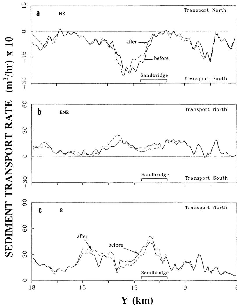
Figure 10. Comparison of longshore sediment transport rates before (solid line) and after (dashed line) the modeled dredging at Sandbridge Shoal for the severe sea ( $H = 3$  m,  $T = 14$  sec) coming from (a) NE; (b) ENE; and (c) E.
