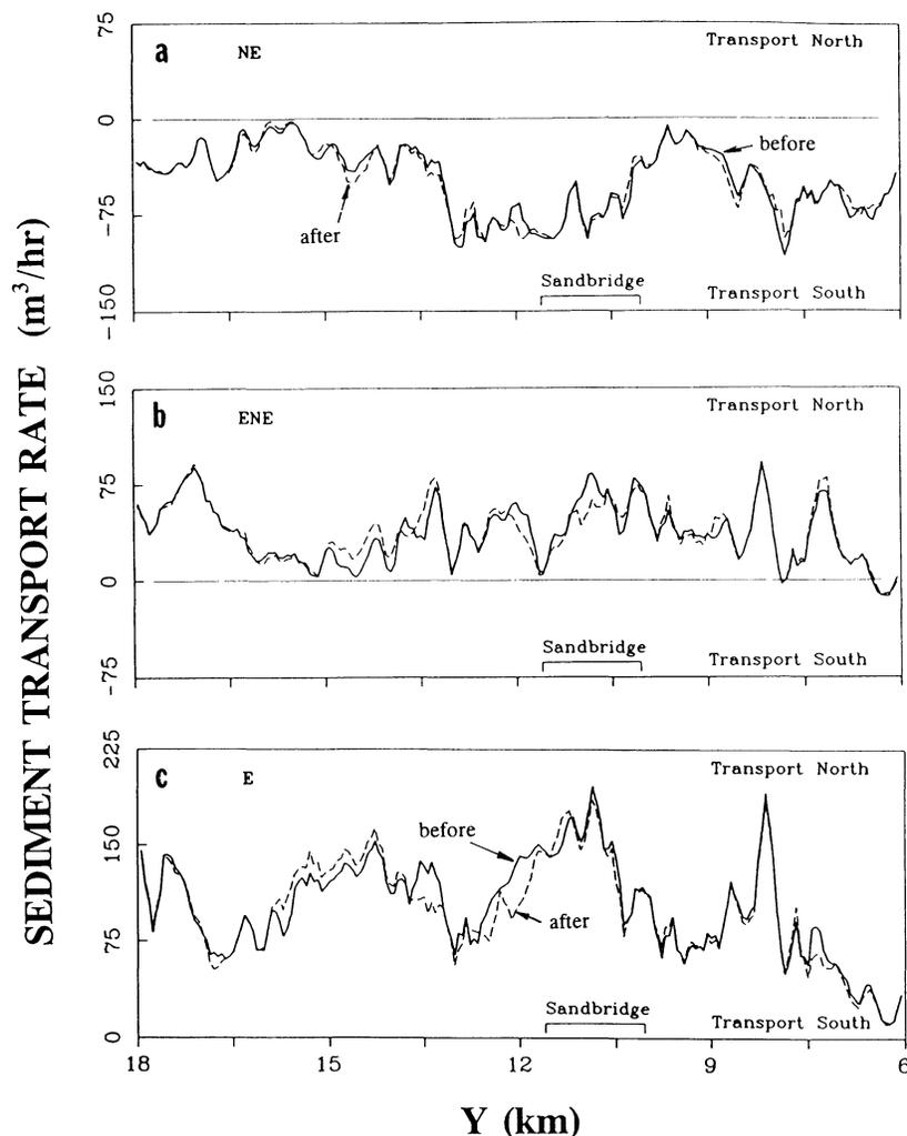
Figure 9. Comparison of longshore sediment transport rates before (solid line) and after (dashed line) the modeled dredging at Sandbridge Shoal for northeaster waves ( $H = 1.9$  m,  $T = 11.8$  sec) coming from (a) NE; (b) ENE; and (c) E.
