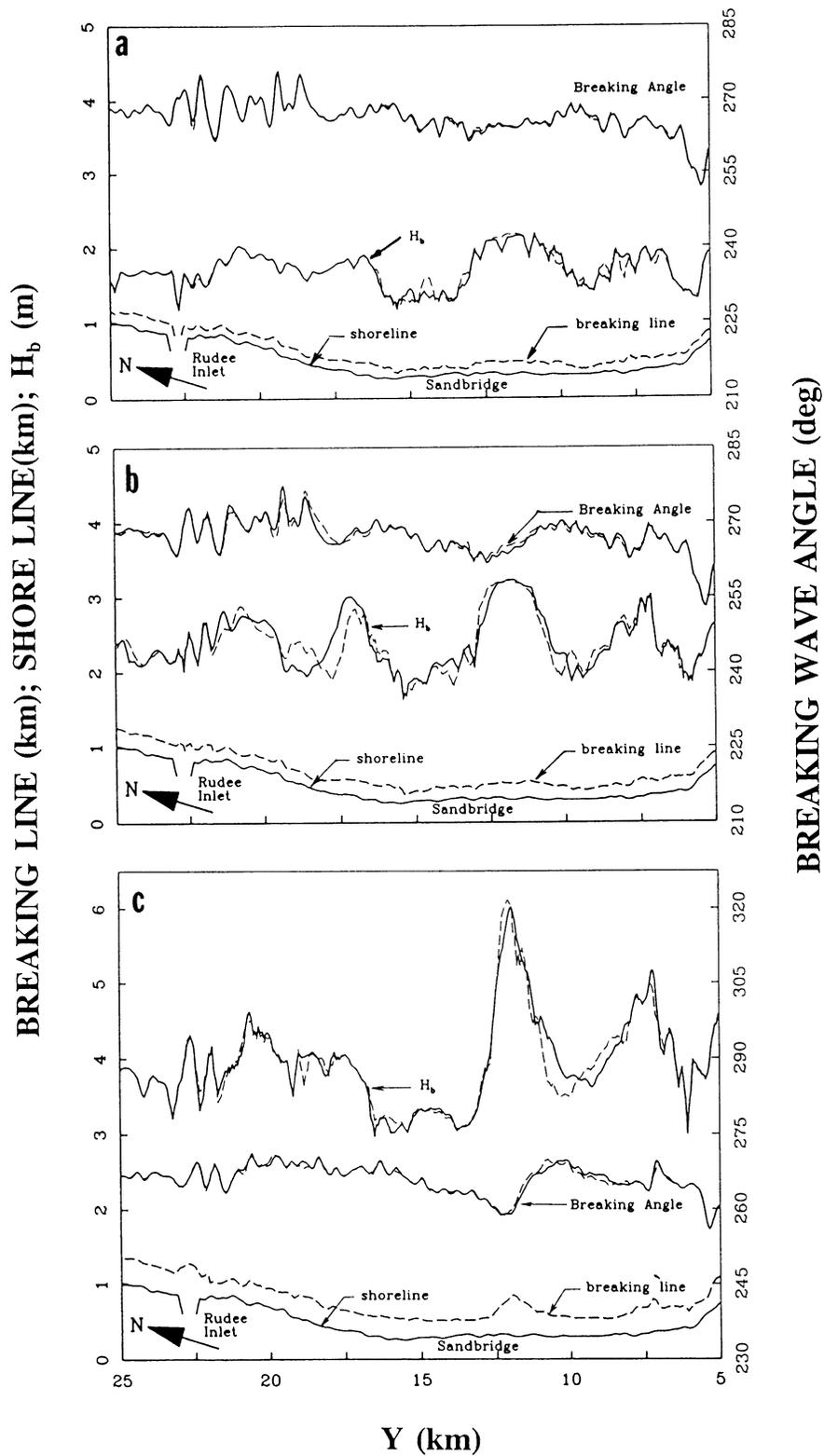
Figure 8. Comparison of breaking wave heights and angles before (solid lines) and after (dashed lines) the modeled dredging for three waves coming from NE. (a) Northeaster waves,  $H = 1.9$  m,  $T = 11.8$  sec; (b) The Severe Sea,  $H = 3$  m,  $T = 14$  sec; (c) The Most Severe Sea,  $H = 6.2$  m,  $T = 20$  sec.
