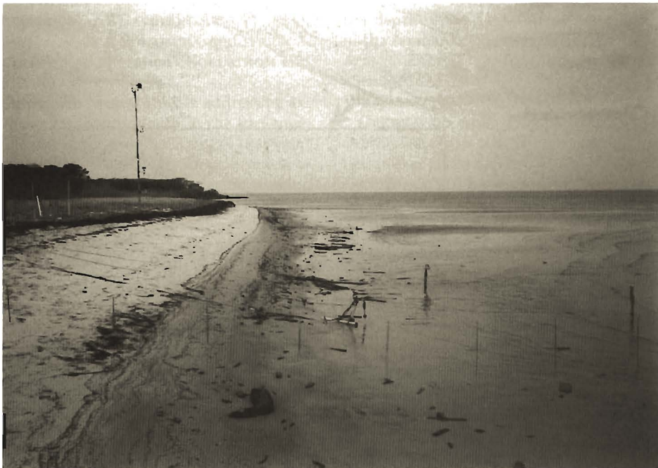
Figure 2. Study site at low water. Anemometer tower is at upper left; survey pins extend across foreground. The pressure transducer used to gather the wave data is mounted on the instrument stand visible near center photo.
