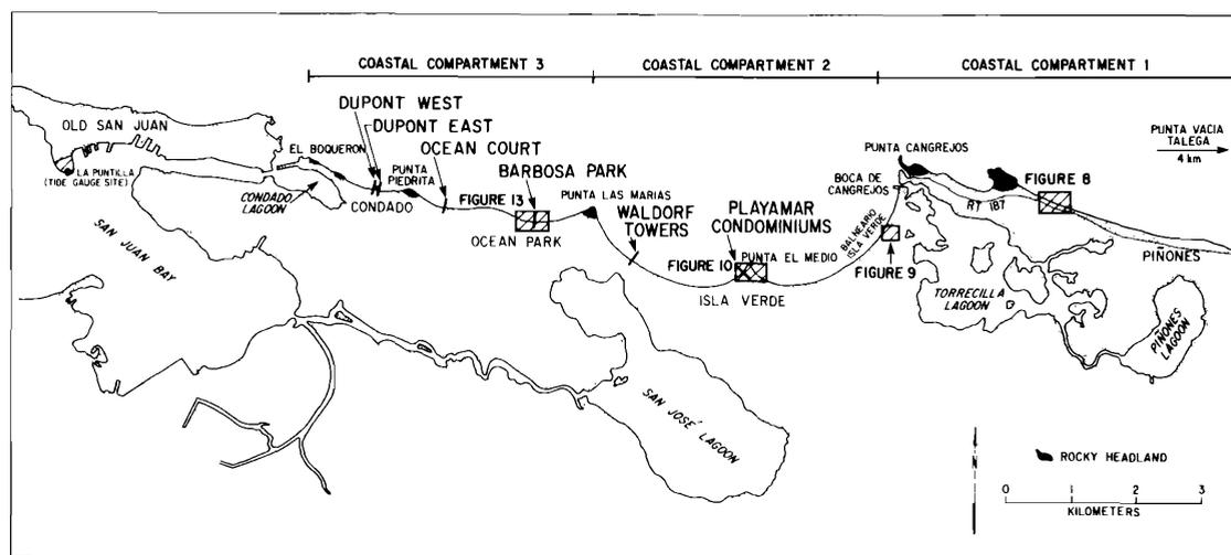
Figure 2. San Juan metropolitan area and coastal compartments. Also shown are locations of aerial and other photographs (Figures 8, 9, 10, and 13). Heavy lines perpendicular to shore are locations of beach profile sites discussed in text.
