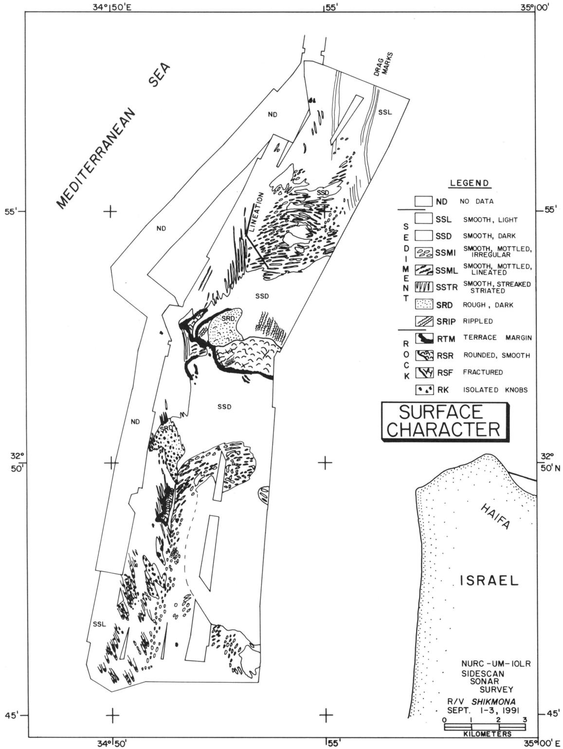
Figure 4. Side-scan sonar map of the Haifa, Israel outer shelf. EG&G SMS 260 digitally rectified images at 200-, 300- and 400-m scales, GPS navigation. Areas not covered by overlapping areal coverage indicated by blank polygons. Line SM-91-1-2 and SM-91-23 were primarily in water too deep for the length of cable available, thus returned no useable data (ND). Note the fractured terrains on the western side of the rocky terraces. Refer to Figure 3 for tracklines.
