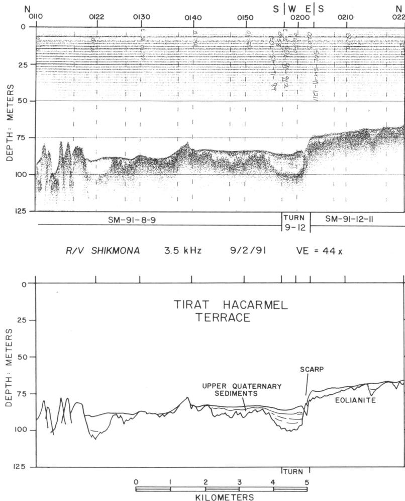
Figure 8. 3.5 kHz seismic reflection profile showing rugged morphology of eolianite subcrops in the Tirat HaCarmel Terrace, smoothed by sedimentary cover. Note the 15 m depth of sediment cover in some places. The step at 90 m depth corresponds to a turn in the line, but also reflects a terrace scarp. Location indicated in Figure 3.
