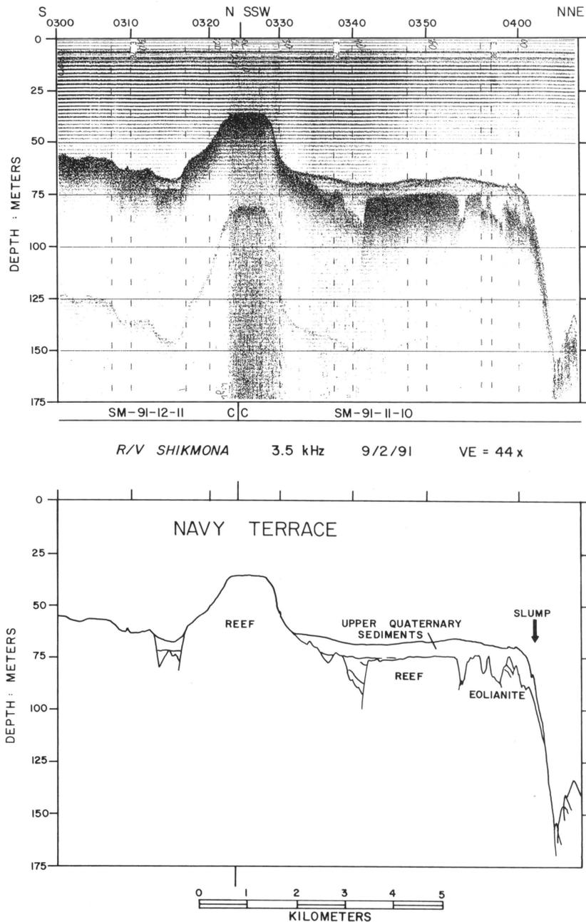
Figure 7. 3.5 kHz seismic reflection profile over the northern margin of the Navy Terrace. This faulted escarpment shows a steep drop of more than 75 m. Slumps and landslides are indicated by the detached block at the top of the escarpment (arrow) and the accumulated sediment at the foot of the slope. Location indicated in Figure 3.
