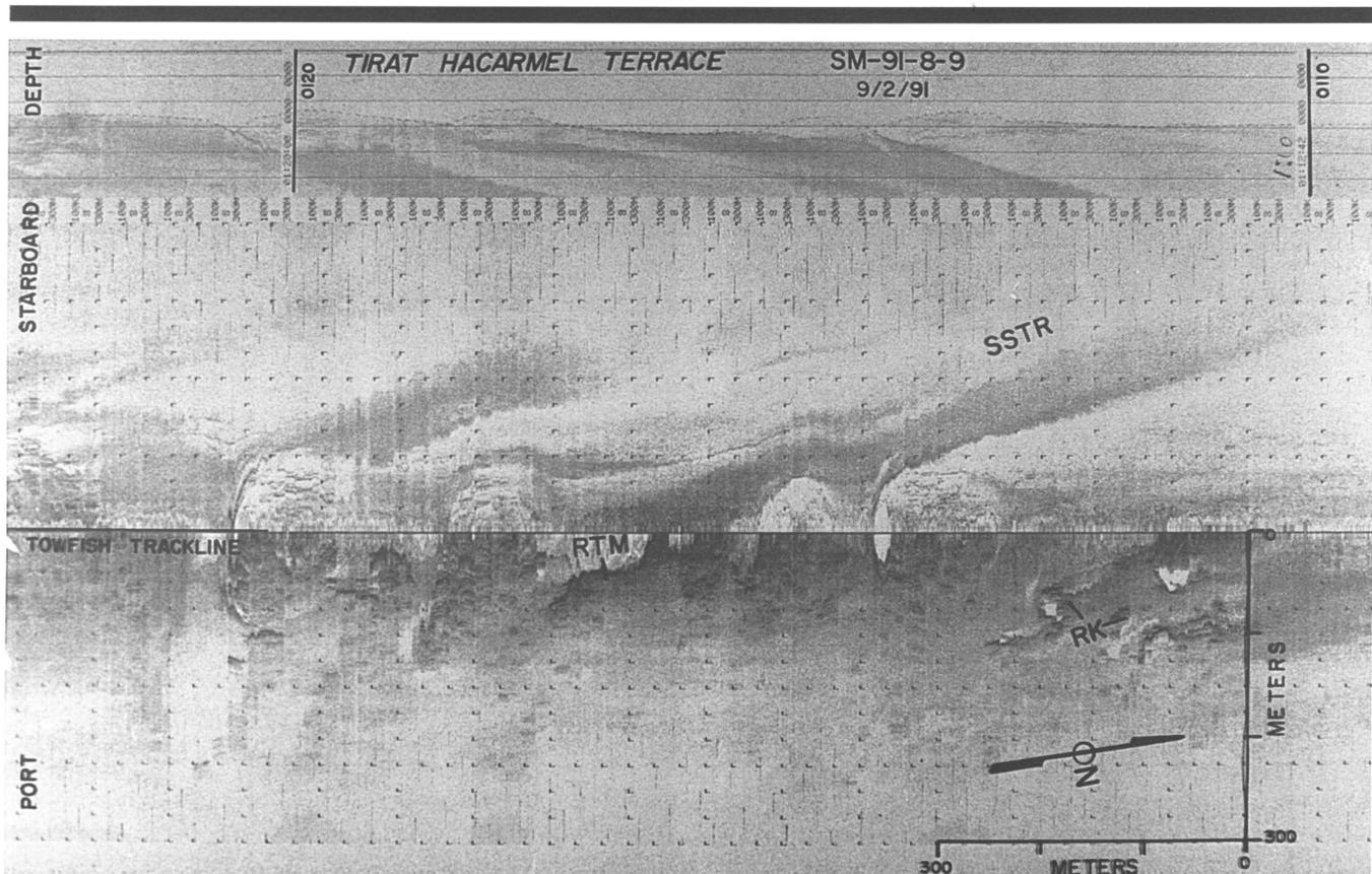
Figure 10. Side-scan sonar image of the Tirat HaCarmel Terrace, with outcrop of subdued relief, and scour marks that indicate NNW flowing bottom currents. Location indicated in Figure 3. Abbreviations for surface character explained in Figure 4.
