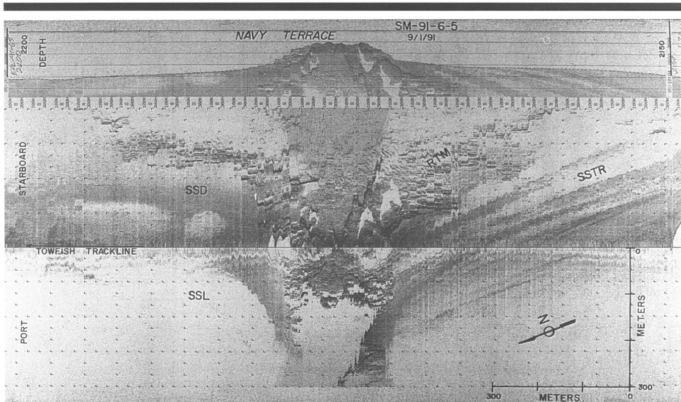
Figure 9. Side-scan sonar image of rocky outcrops of the Navy Terrace. Note the west-facing cliffs along many of the ridges. Location indicated in Figure 3. Abbreviations for surface character explained in Figure 4.
