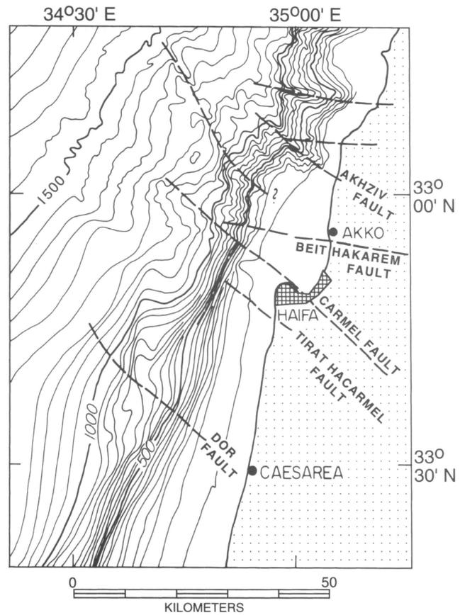
Figure 2. Bathymetric map of the Carmel Promontory and Haifa Bay, after Hall (1980). Heavy lines indicate major faults (Mart, 1984). Note the orthogonal pattern of faulting off Haifa.
