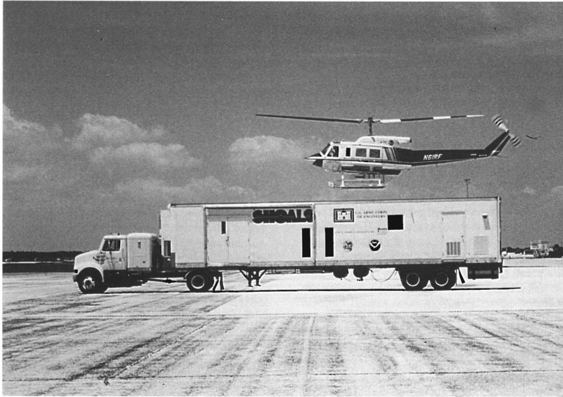
Figure 2. SHOALS helicopter and mobile field unit. The mobile unit provides the capability to process and output the lidar survey data while on site.
