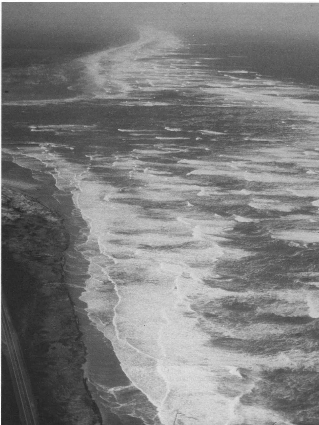
Oregon Inlet, North Carolina. View looking north on 31 October, 1991 during the height of the "Halloween" storm. The ebb shoal is well defined by the rare (for the east coast) 5 m, 22 sec waves. Oregon Inlet, which separates Bodie Island (above) from Pea Island, opened in 1846 almost 4 km north of its present position where the shoreline is offset (background) to the west. (Photograph by Carl Miller, WES/CERC Field Research Facility, Duck, North Carolina).
