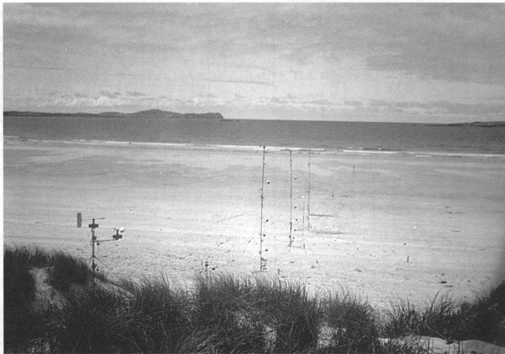
Plate 1. Study site during field deployment. Anemometers on the masts with wind vanes in the foreground did not function properly during the experiment.
