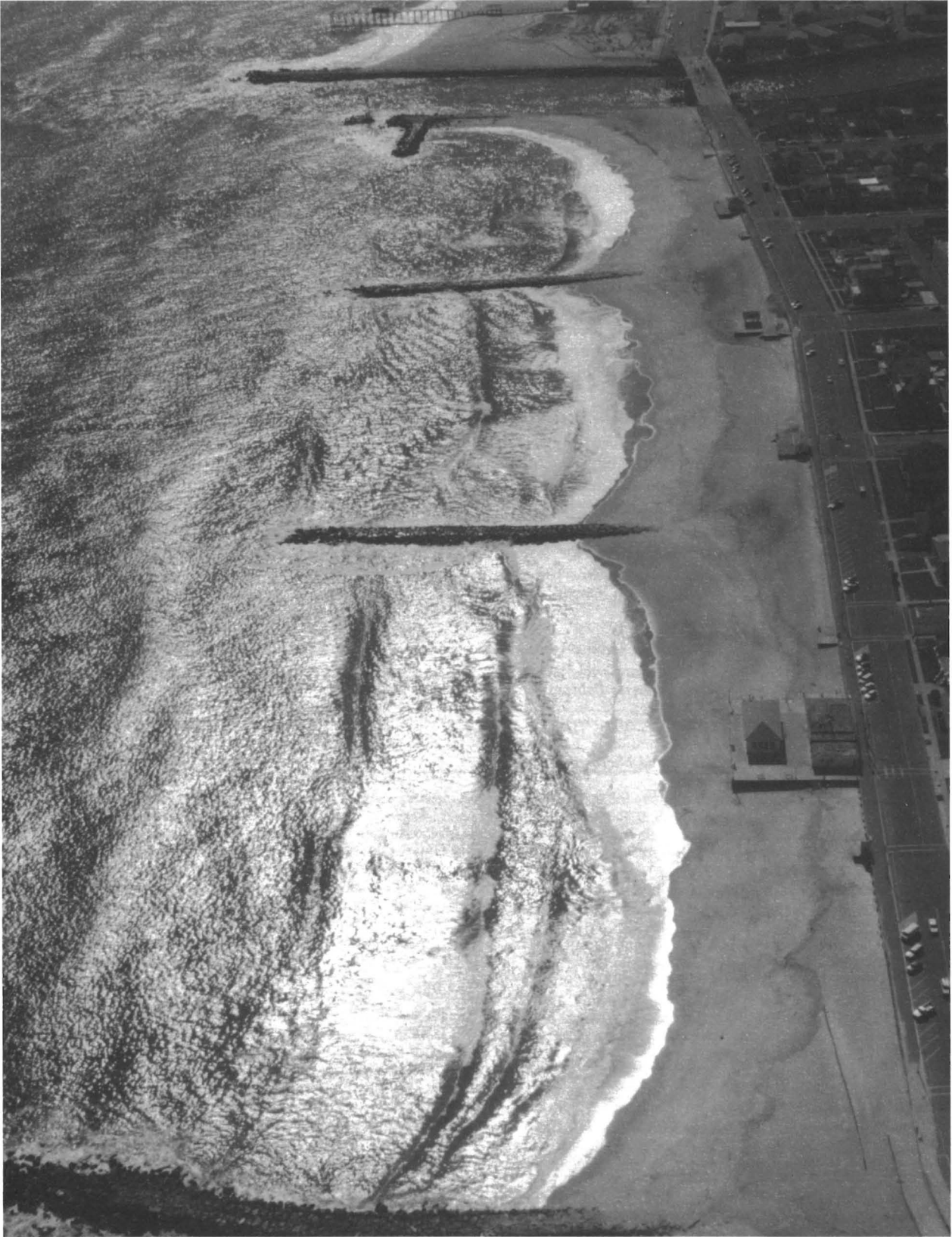
Coastal processes, Monmouth County, New Jersey. Looking south from Avon, across Shark River Inlet, toward Belmar, New Jersey, at 1245 pm, 18 Oct 94. The ocean tide is about 1.3 hr past predicted low, but the bay tide is just about at predicted low and still ebbs out the inlet. Atlantic waves on the low tide terrace between the Avon groins travel shoreward as solitons, and reflect seaward from the foreshore as higher frequency waves. The nearer inlet jetty has a gap caused during the great northeaster of 11 Dec 92, possibly by waves converging between the rock spur and the jetty tip and overtopping into the inlet. The navigation light on the now-isolated tip of this jetty survived that storm and still operates, but the light on the opposite jetty was torn up with its concrete foundation and thrown back on Belmar beach. Net longshore transport direction is clearly toward the viewer, from south to north. This area is within the limits of planned Corps of Engineers beach fill. (Photograph by Cyril Galvin, Coastal Engineer, Box 623, Springfield, Virginia 22150, USA).
