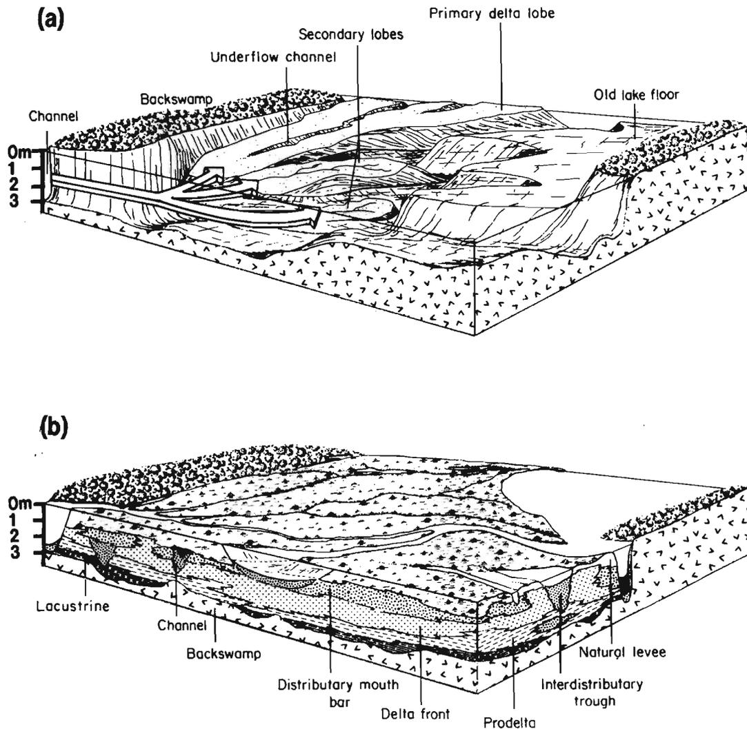
Figure 5. Schematic representation of lacustrine delta evolution illustrating (a) morphology of elongate lobes characteristic of these delta types and (b) sedimentary architecture of a fully developed delta (modified from Tye and Coleman, 1989).
