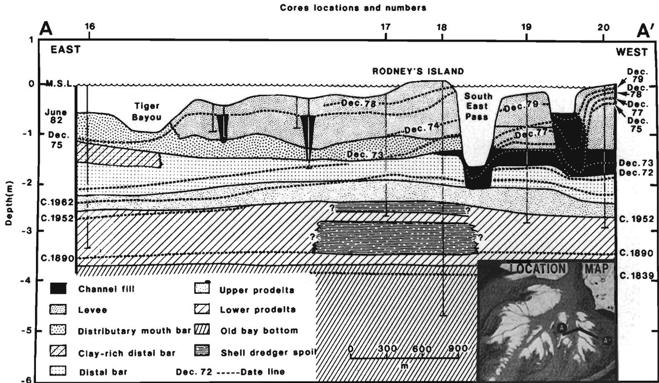
Figure 10. Stratigraphic cross section from the eastern sector of the Atchafalaya delta as prepared from a vibracore transect. Coring sites are designated on the cross section (modified from van Heerden, 1983). Chronostratigraphic surfaces determined by historical bathymetry of Atchafalaya Bay and surveyed profiles across the delta.
