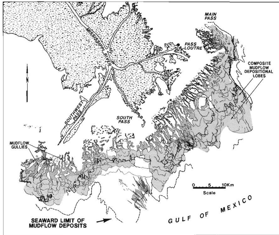
Figure 17. Distribution of mud flow gully systems and their associated down-slope deposits (modified from Coleman *et al.* 1980).
