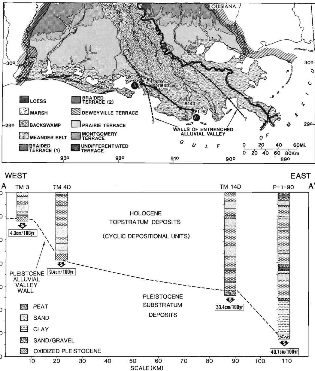
Figure 20. (Top) Map of the Mississippi River deltaic plain and southern alluvial valley showing the approximate position of the entrenched alluvial valley beneath delta plain deposits and the location of borings and cross section. (Bottom) A west-to-east transect of borings showing the influence of Holocene sediment thickness on subsidence rates as determined from  $^{14}\text{C}$  dates (modified from Roberts *et al.*, 1994).
