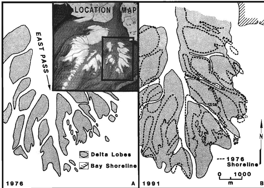
Figure 9. Comparison of sedimentary lobes in the eastern Atchafalaya delta (1976–1991) illustrating the process of lobe fusion and upstream accretion of sand-rich deposits.
