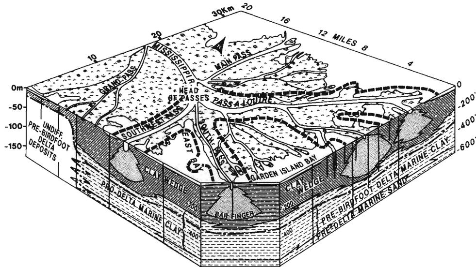
Figure 13. Block diagram of elongate distributary mouth bar sands, or bar-finger sands (Fisk, 1961), illustrating the elongate sand trends that develop in river-dominated deltas prograding into deep water (modified from Fisk *et al.*, 1954).
