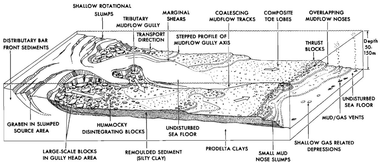
Figure 18. Block diagram showing the salient components of a retrogressive mudslide system typical of the Mississippi River delta front. The system has been greatly shortened for illustration purposes (Roberts *et al.*, 1980). Length to width ratios of these mudslide systems are 20–30:1.
