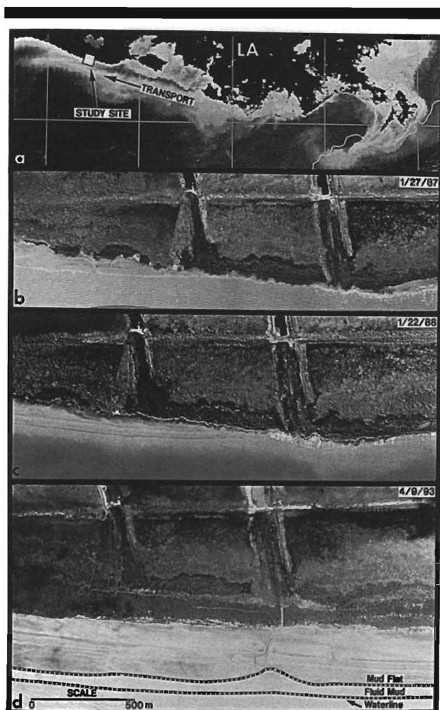
Figure 11. A series of photographs of the eastern chenier plain coast illustrating rapid progradation between 1987 and 1993. In this sector of the coast, average progradation rates were about 50 m/yr during this period. Fine-grained sediments supplied by the Atchafalaya River are responsible for these dynamic coastal changes.
