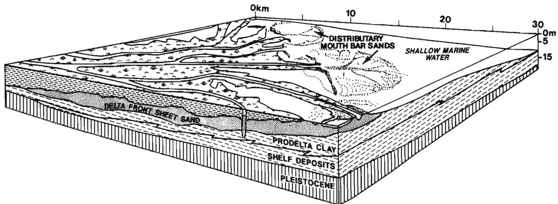
Figure 14. Block diagram depicting a delta front sheet sand associated with the numerous and closely spaced distributaries of a thin inner shelf delta, such as the Lafourche delta (modified from Fisk *et al.*, 1954).
