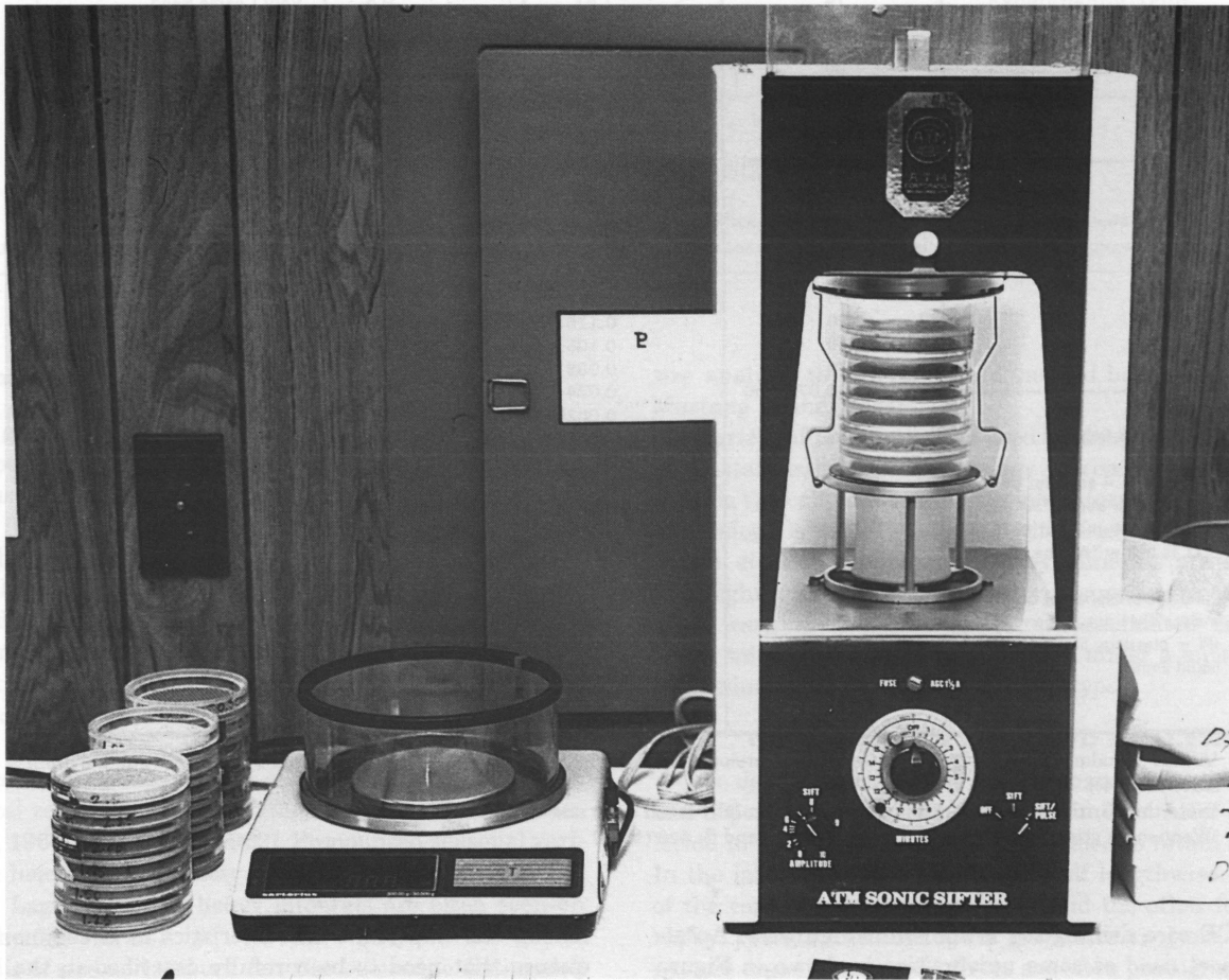
Figure 9. Gilson GilSonic sonic sifter and balance used with 1/4 \phi sieves for grain size analyses.
