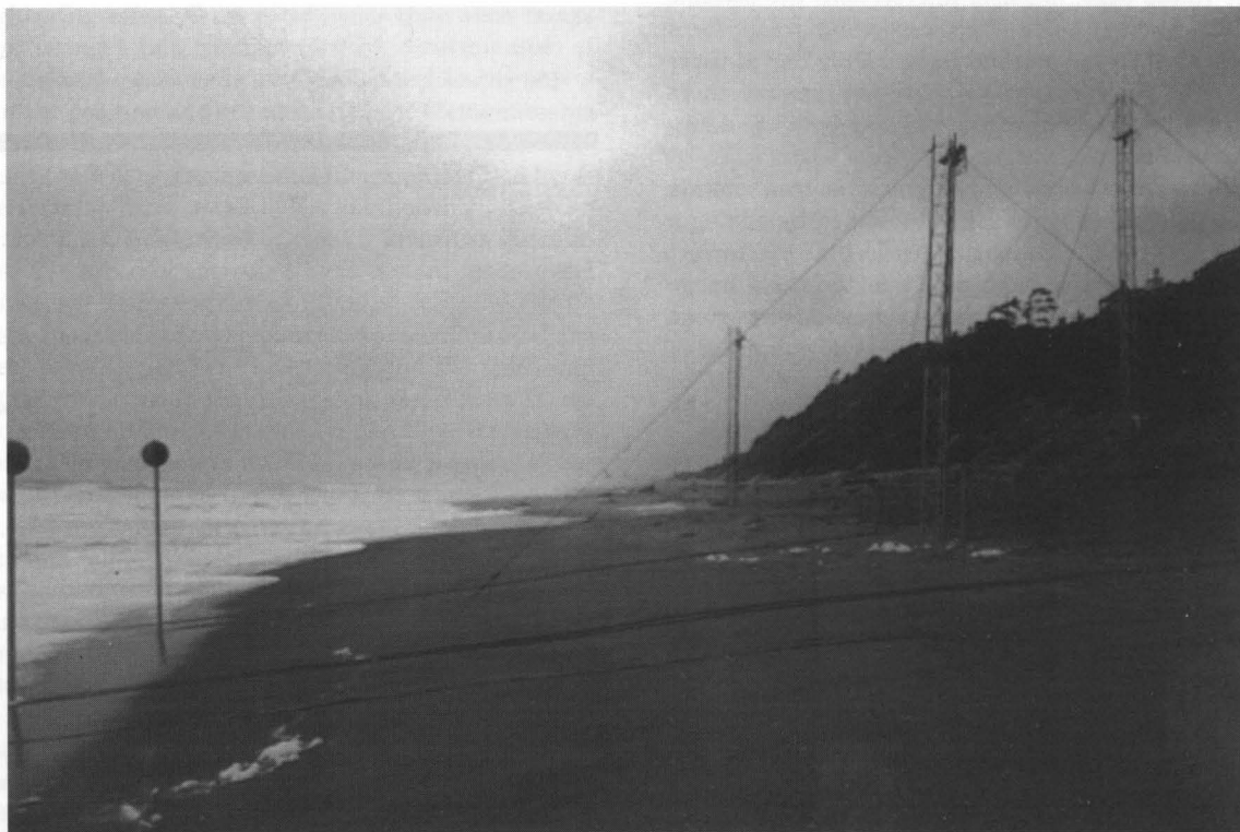
Figure 5. Photograph of the field experiment showing video camera housings mounted on radio antenna towers. The circular objects on the foreshore are permanent ground control points.
