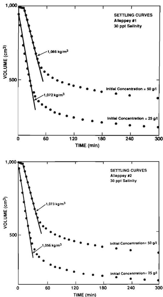
Figure 2. Hindered settling curves for the two Alleppey samples, settled at 25 and 50 g/l in water of 30 ppt salinity. Linear settling changes at suspension density of 1,073 kg/m<sup>3</sup> in all samples, indicating structural formation associated with hindered settling occurs at that density: (a) Settling of Alleppey #1, (b) Settling of Alleppey #2.
