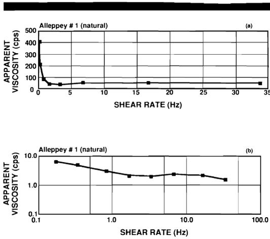
Figure 4. Rheogram of the natural bed sediment at Alleppey #1. The sample demonstrates a continuous reduction in 'apparent' viscosity to a shear rate of approximately 5 Hz. Shear thickening occurs between 5 and 7 Hz and is followed by shear thinning to 34 Hz (a). This behavior is also shown on a log-log scale in (b).
