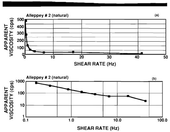
Figure 5. Rheogram of the natural bed sediment at Alleppey #2. The sample shows a nearly continuous reduction in 'apparent' viscosity. An indication of Newtonian flow occurs at about 18 Hz and is followed by shear thinning to 42 Hz (a). This behavior is also shown on a log-log scale in (b).
