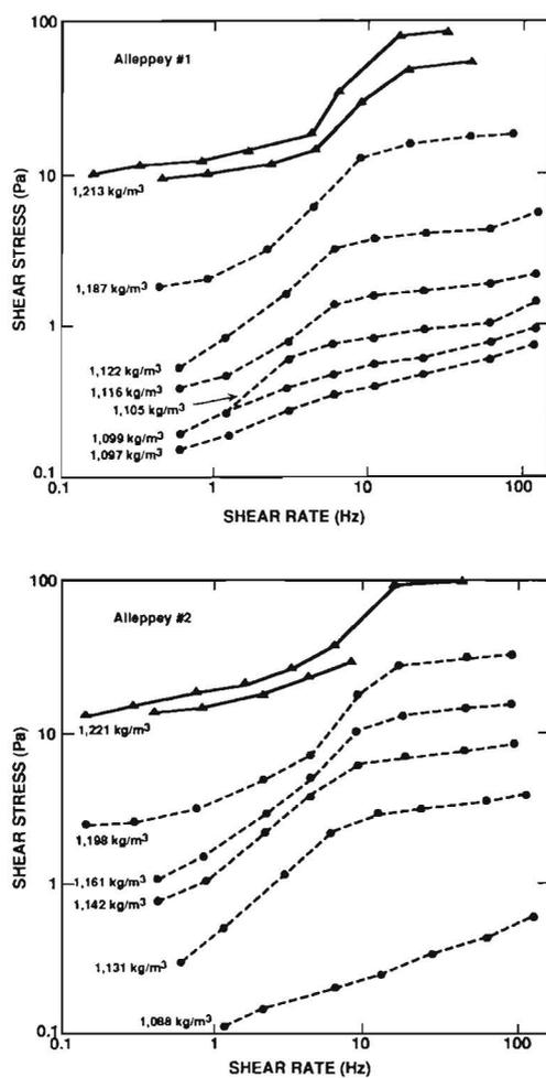
Figure 3. Flow diagrams for the two Alleppey samples, each showing the flow behavior of the undisturbed sediment bed (solid lines) and the resuspended sediment at different sample densities (broken lines): (a) Flow behavior of Alleppey #1, (b) Flow behavior of Alleppey #2.
