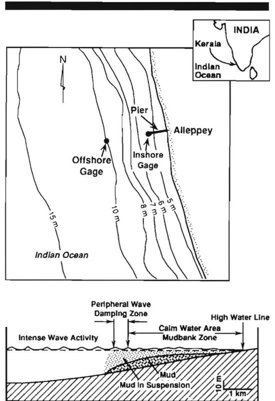
Figure 1. a. Position of pier and nature of bottom topography off Alleppey, Kerala, India. The distance between the offshore wave gage and the inshore wave gage is 1.1 km. b. Schematic profile of a mudbank region (after NAIR, 1988).
