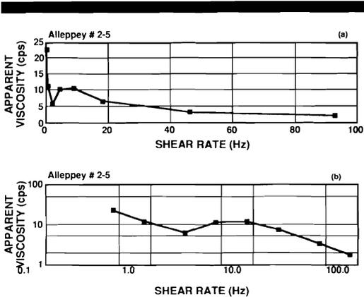
Figure 7. Rheograms of Alleppey #2-5 (density 1,161 kg/m<sup>3</sup>), a suspension made from a bed sample from Alleppey #2. a) shows clearly the apparent viscosity increase (shear thickening) which occurs between 2 and 5 Hz. This is followed by an interval of constant apparent viscosity (Newtonian flow) to 9 Hz. The remainder of the figure shows apparent viscosity decreasing (shear thinning) to the end of the shear rate scale. b) shows the same data on expanded logarithmic coordinates.
