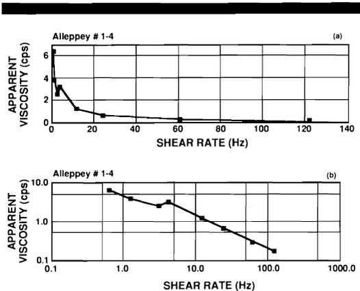
Figure 6. Rheograms of Alleppey #1-4 (density 1,118 kg/m<sup>3</sup>), a suspension made from a bed sample from Alleppey #1. a) shows clearly the apparent viscosity increase (shear thickening) which occurs between 3 and 6 Hz. Apparent viscosity continues to decrease to the end of the run after 6 Hz. b) shows the same interval of apparent viscosity increase (shear thickening) on expanded logarithmic coordinates.
