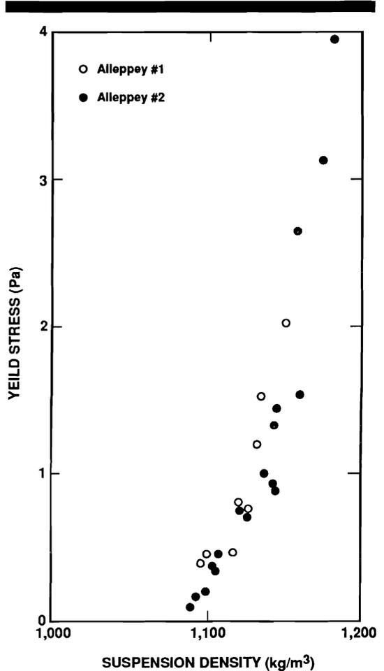
Figure 8. Plot of yield stress (measured at lowest possible shear rate) versus suspension density for both Alleppey #1 and Alleppey #2 samples.
