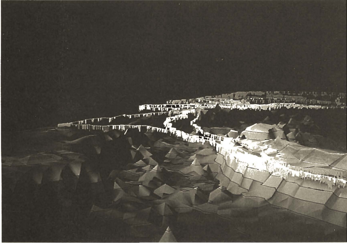
Figure 3. The diving pattern (vertical lines) and track (horizontal line) of 10 Elephant Seals, shown in relation to ocean bathymetry off South Georgia Island. The track was obtained using an ARGOS satellite-linked time depth recorder attached to each seal. This provided accurate data which was then input to a GIS for subsequent analysis and presentation. Source: The Oceanography Society (1993) (courtesy of Sea Mammal Research Unit, NERC, U.K.).
