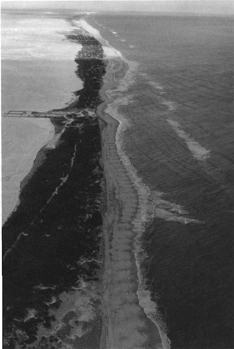
Erosion Wave on Fire Island, New York. Aerial photograph, view east of Fire Island, off of the Atlantic Ocean coast on the South Shore of Long Island. An erosion wave is located along this section of shoreline near Water Island. Note the sinuous nature of the shoreline, the symmetry of the feature and the relationship of the offshore sandbar system. The entire erosion feature has been slowly migrating to the west over the past 8 months. (Photograph by Dan Covello, 15 January 1994).
