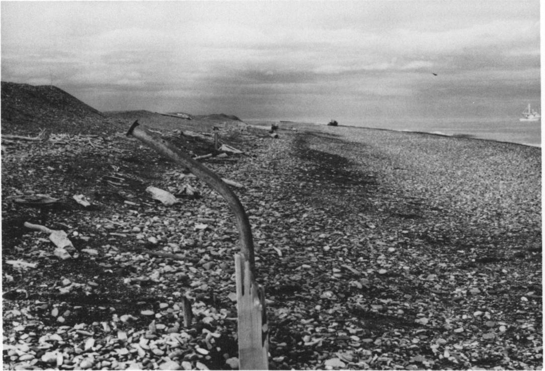
Figure 15. The triangulation station EASY, with 4×4 inch witness post and bent reference mark in foreground, on the beach about 1 m below the modern crest of Icy Reef (1987). The island apparently was elevated by about 1 m through gravel stacking by pile-ups since 1952.
