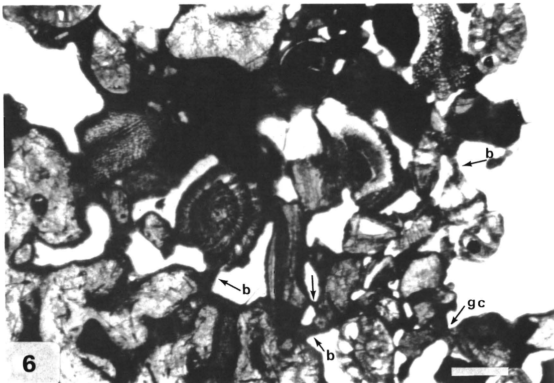
Figure 6. Typical marine vadose matrices from the upper sequence of exposed rubbly deposits on St. Joseph Atoll (sample RS 1.50, collected at +0.45 m above present MSL): occurrence of scattered patches of dense micrite matrix, laterally changing into thin rims in a grain-contact attitude (gc) or in the form of bridges between adjacent grains (b). (Scale = 100 \mu m).
