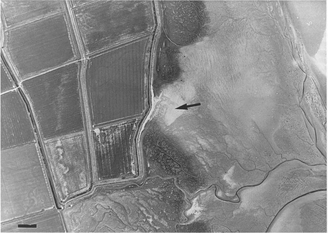
Figure 10. Vertical air photograph taken in 1989 showing erosion of the saltmarsh and mudflats (arrowed) in front of the 1979 embankment at Butterwick in the southwestern part of the Wash. Scale 1:10,000. Reproduced by permission of the Aerial Photography Unit, Cambridge University.
