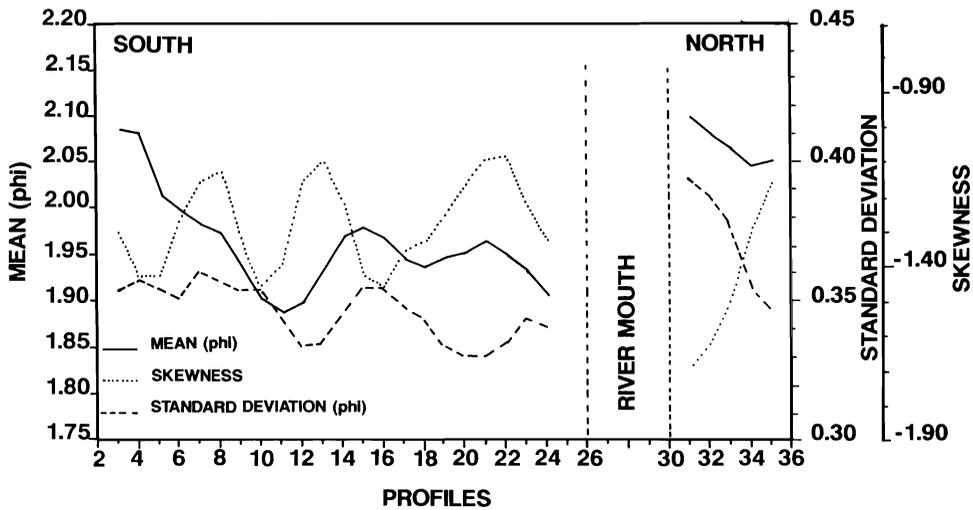
Figure 7. Longshore textural parameters distribution (mean grain size, standard deviation and skewness).
