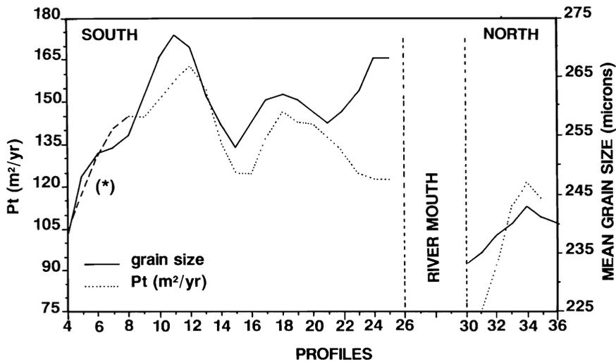
Figure 13. Wave power and mean grain size along the Ebro Delta coast (\*: portion of the curve induced from coastal orientation, not used in the analysis of correlation).
