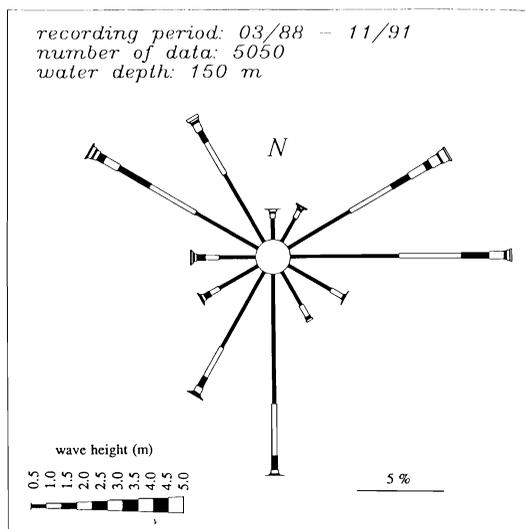
Figure 2. Offshore wave height directional distribution at the Ebro Delta coast (JIMENEZ *et al.*, 1992).
