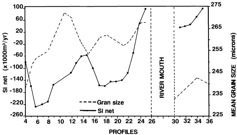
Figure 10. Net longshore transport rates and mean grain size along the Ebro Delta coast (negative values indicate a southward transport; note—profiles are not equidistant).
