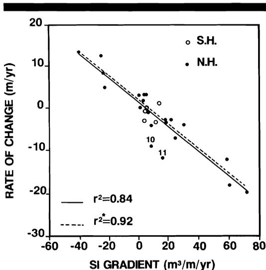
Figure 11. Shoreline rate of change versus longshore transport gradients (\*: without profiles 10 and 11).
