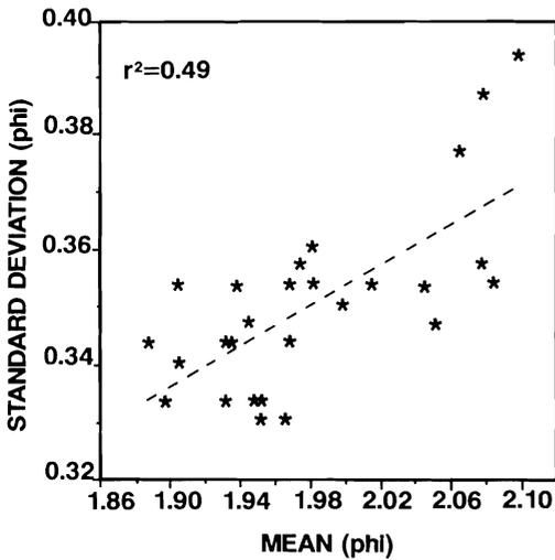
Figure 4. Standard deviation versus mean grain size.
