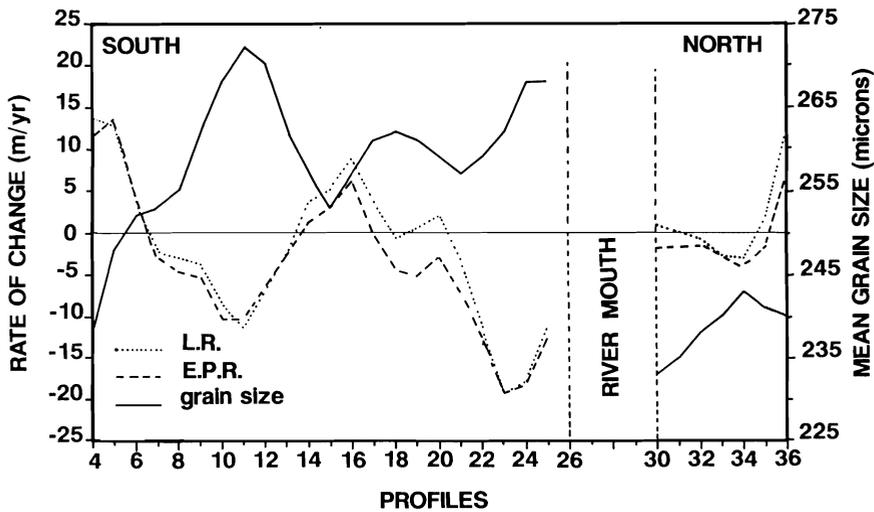
Figure 8. Shoreline rates of change and mean grain size along the Ebro Delta coast (LR: rate obtained using a linear regression technique; EPR: rate obtained using the end-point-rate method). (Microns units are used in what follows for a better visualization.)
