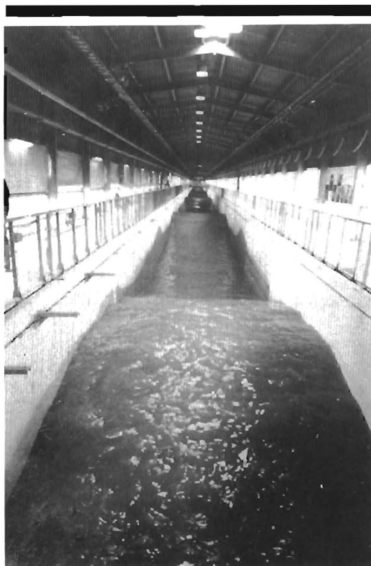
Photo 1: A typical wave generated in the flume (wave height (H ia ): 2.0 m, wave period (T): 10 sec.
