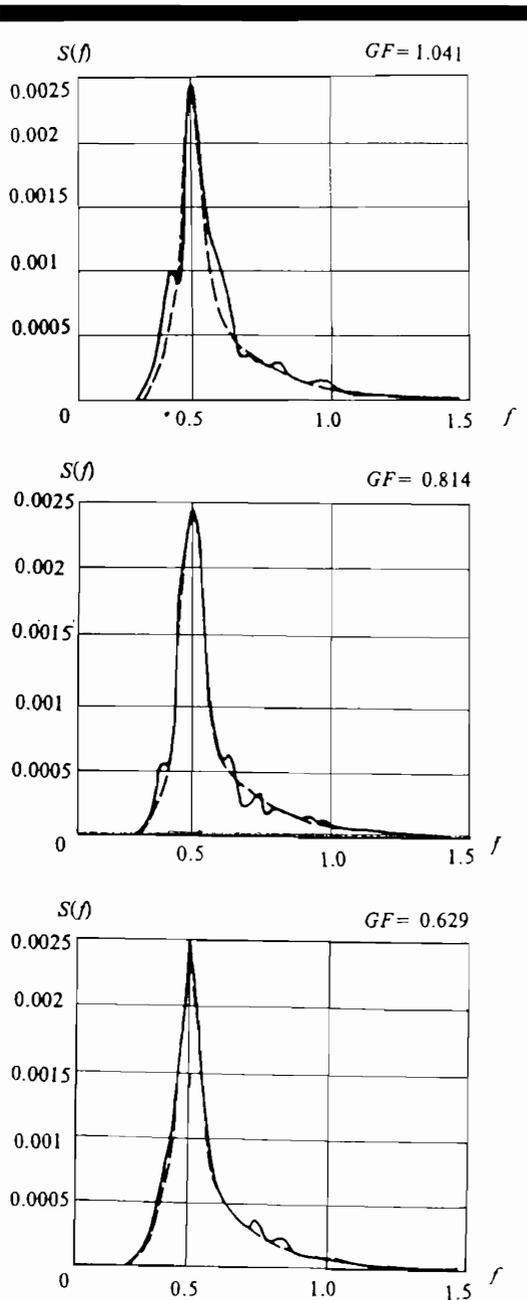
Figure 1. Calibrated curves and theoretical curves for wave spectrum.
