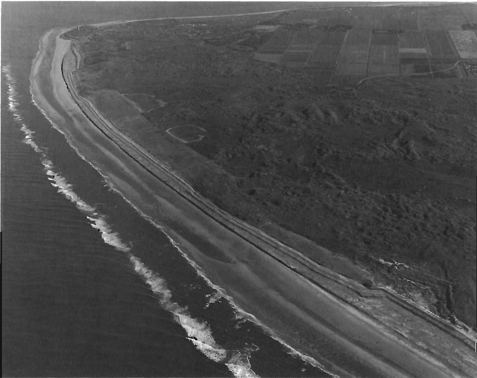
Figure 1. Oblique air photograph of the Wadden island of Texel showing a natural dune landscape cut off by an artificial foredune. (Source: KLM Aerocarto, vogelvlucht fotografie, KO 18187.)
