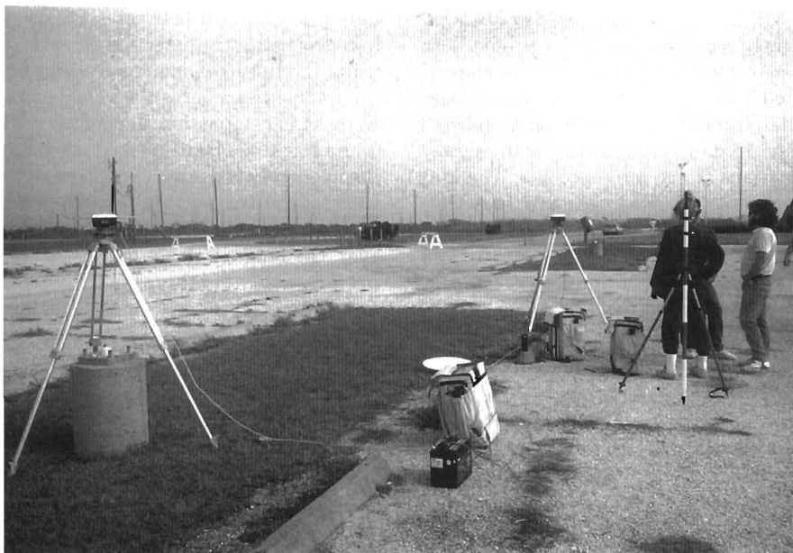
Figure 3. Configuration of GPS equipment at the reference point and index point of the baseline.
