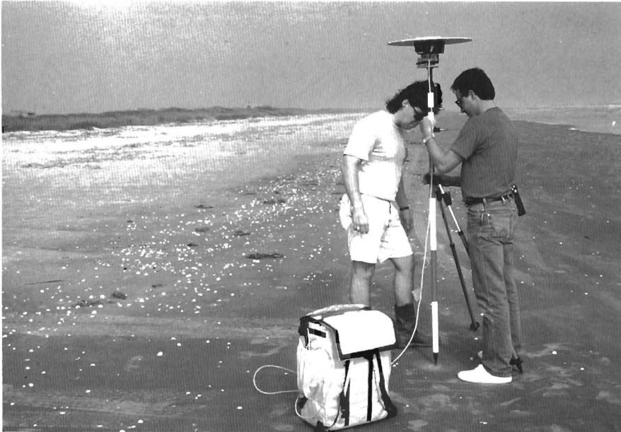
Figure 4. Configuration of GPS equipment during stop-and-go surveys. This procedure is comparable to a conventional land survey whereby static positioning data are collected at discrete stations along a transect.
