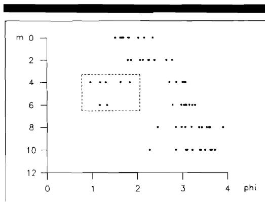
Figure 2. Mz/Depth scatterplot for sediments in the study area. Dashed line encloses points representative of bar sediments.
