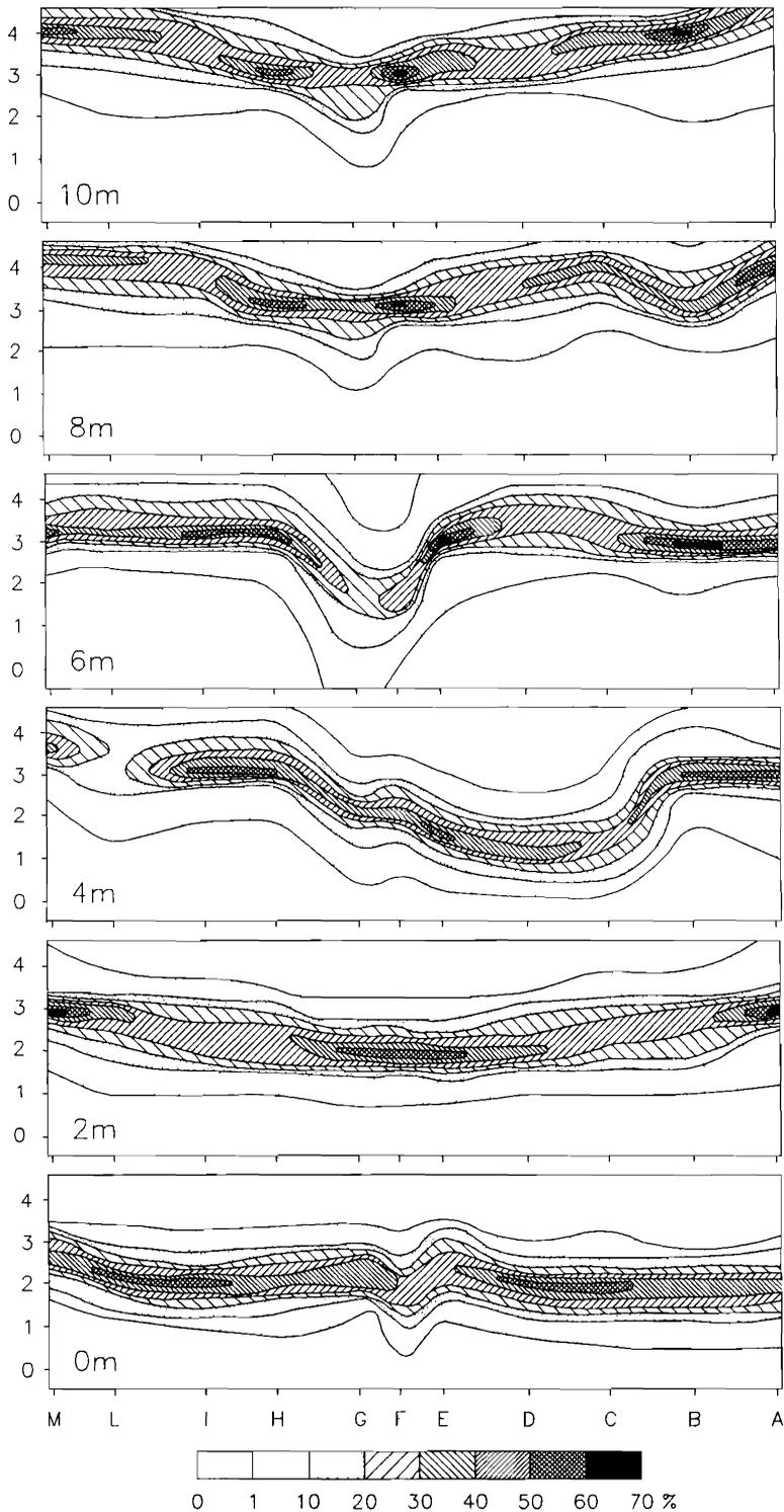
Figure 7. Grain size spectra maps for sediments at different depths.
