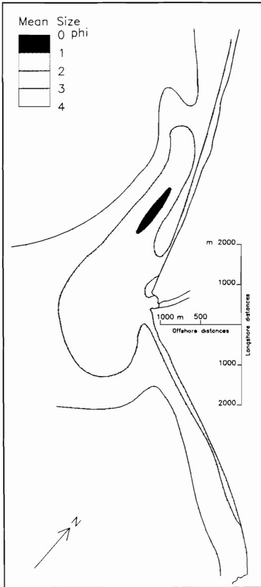
Figure 3. Ombrone River delta: mean size sediment ( $M_z$ ) map. Offshore distances have been doubled for clarity.
