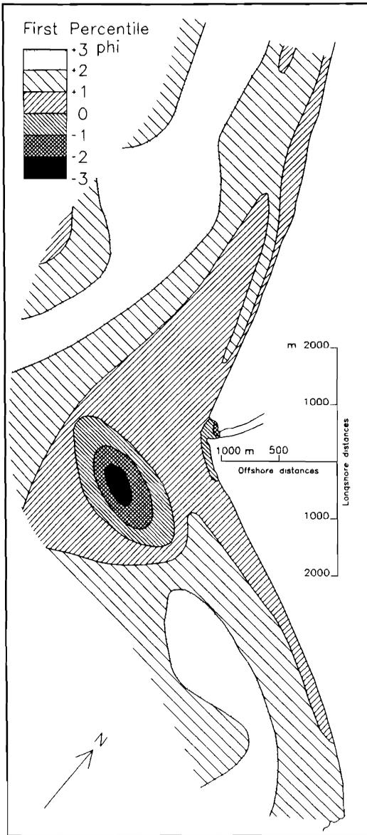
Figure 5. Ombrone River delta: 1<sup>st</sup> percentile size map. Offshore distances have been doubled for clarity.
