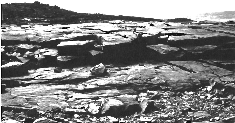
Figure 7. Example of disjunction quarrying along a quarrying front.
