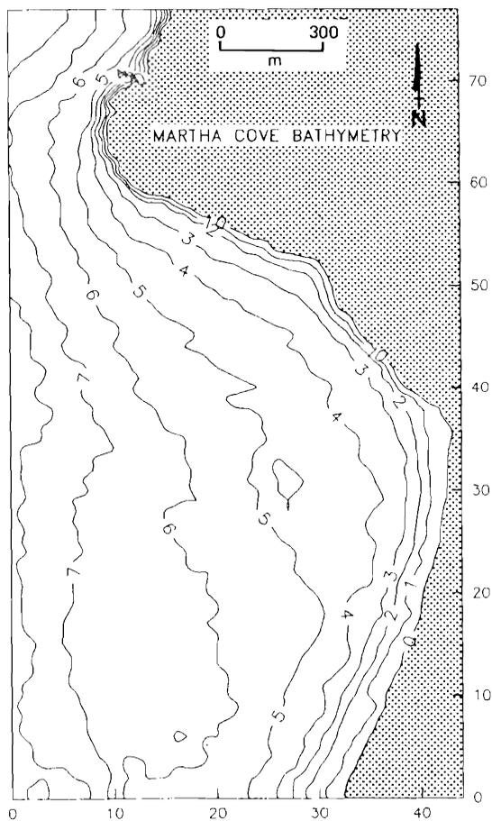
Figure 3. 30 m bathymetry grid showing depths in metres and model cell numbers.
