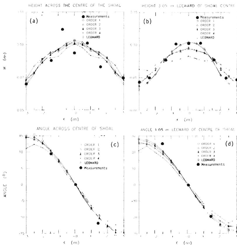
Figure 6. Comparison of wave height and angle predictions with measurements on an elliptical shoal using a variety of y-derivative approximations. (a) Wave height across the centre of the ellipsoid. (b) Wave height 3.05 m leeward of the centre of the ellipsoid. (c) Wave angle across the centre of the ellipsoid. (d) Wave angle 3.05 m leeward of the centre of the ellipsoid.
