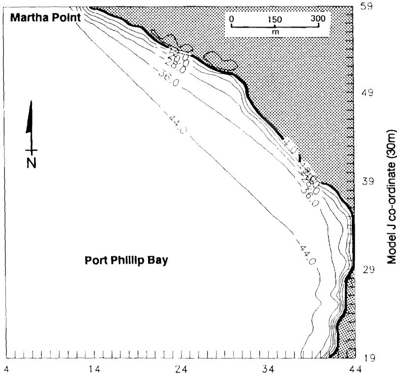
Figure 7. Wave angles in the lee of the headland (relative to due east) for an offshore height of 1 m and angle at 315°T.
