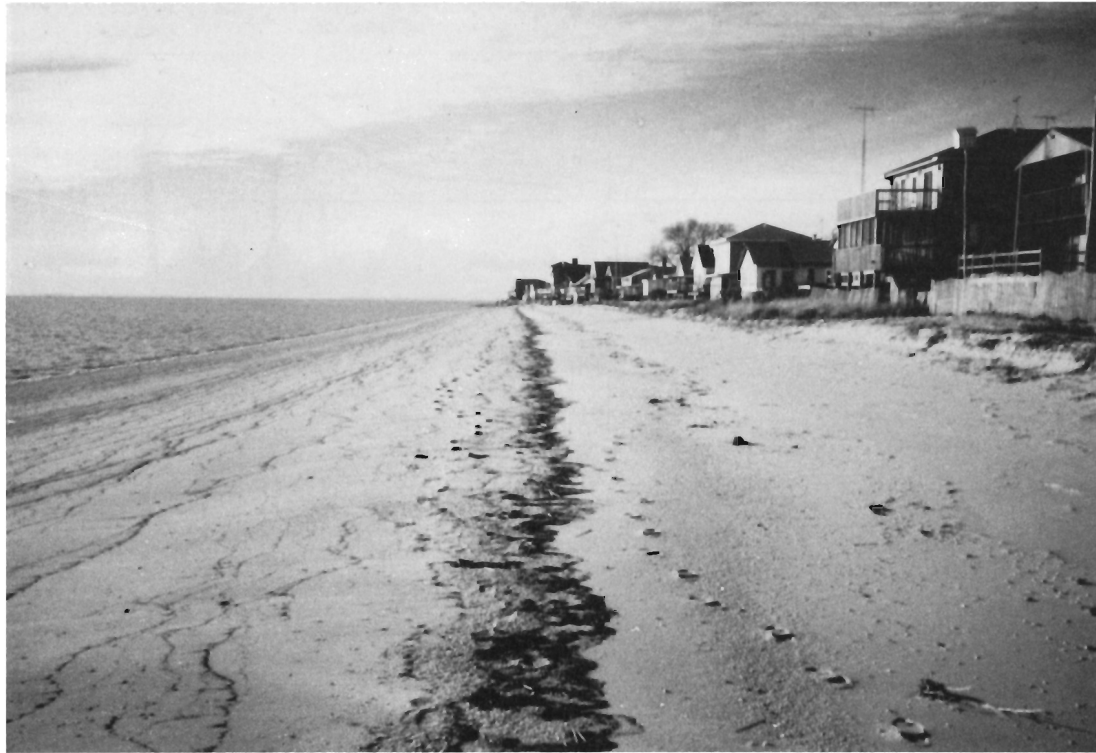
Figure 4. Gandys Beach, New Jersey, in Delaware Bay, facing northwest, showing buildings behind the beach that alter wind flow and lack of shore-perpendicular obstructions to transport.
