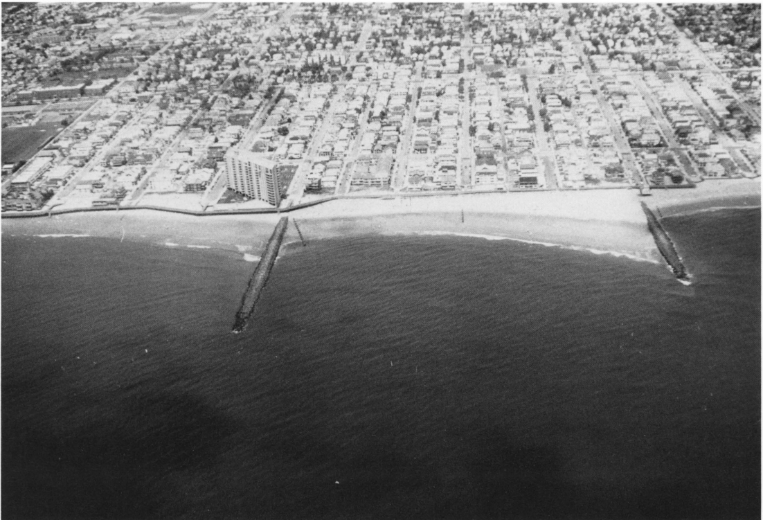
Figure 3. Type II beach with shore parallel structures and a variable beach width due the sand offset by the groins in Ocean City.
