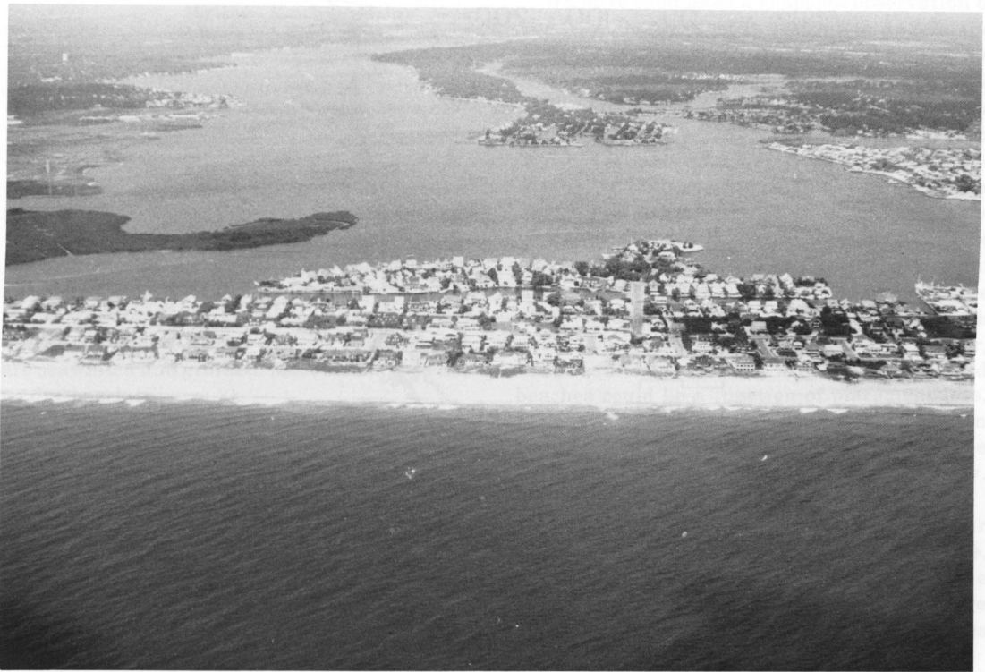
Figure 5. Type IV beach, one with no hard stabilization structures. Note the relatively uniform beach width for the Bay Head area.
