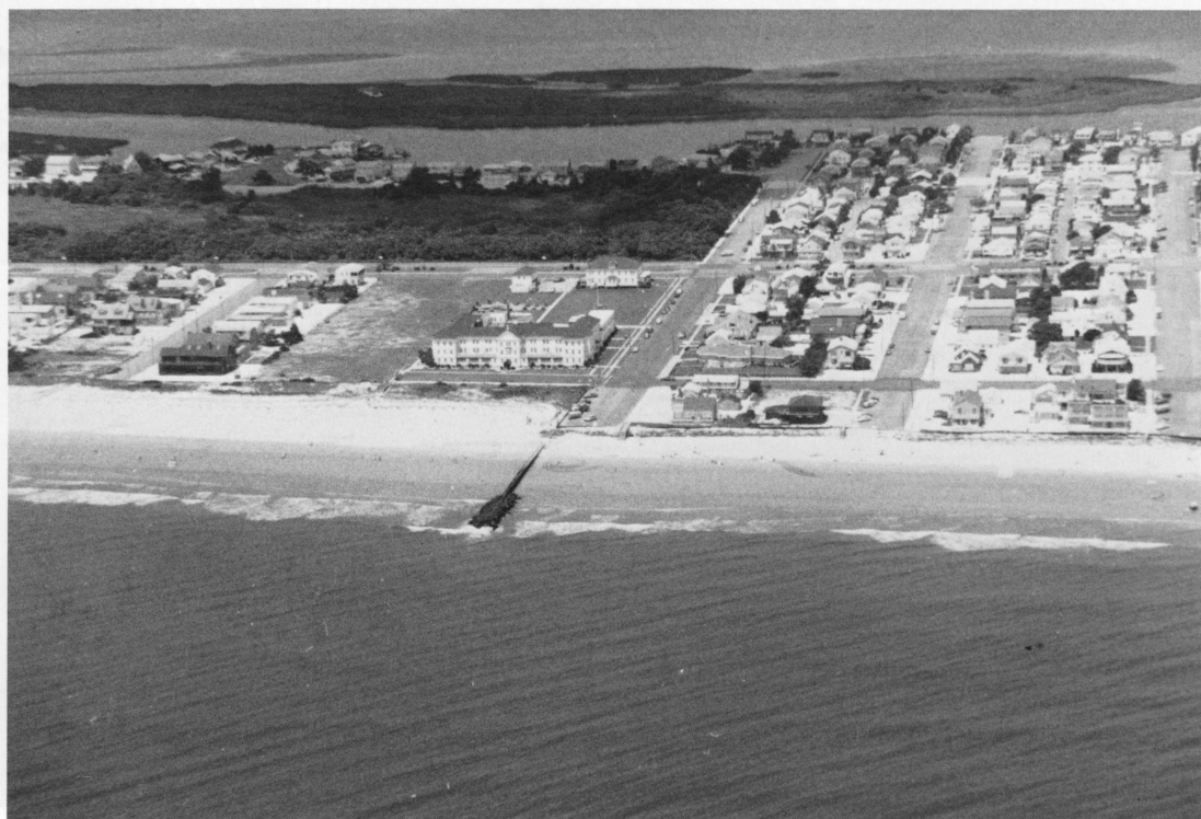
Figure 4. Type III beach, shore perpendicular structure with no offset, as seen in Stone Harbor.
