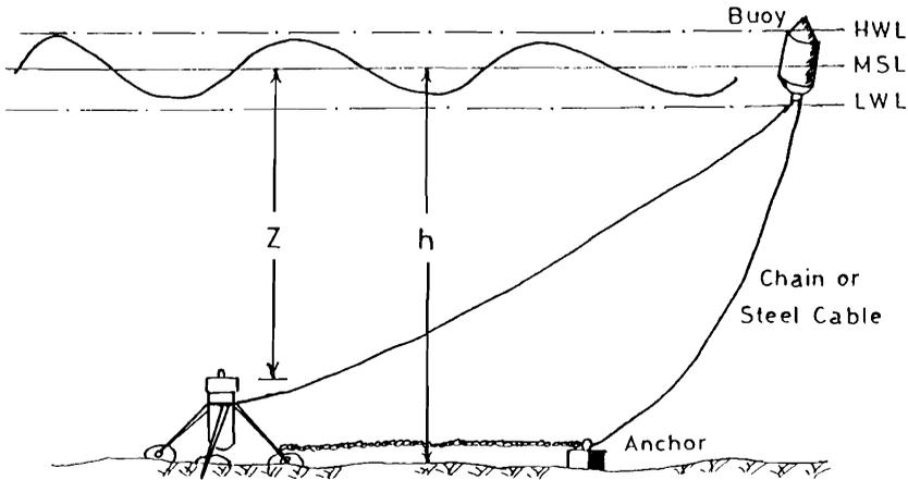
Figure 2a. Arrangement of OSPOS Wave Recorder system.
