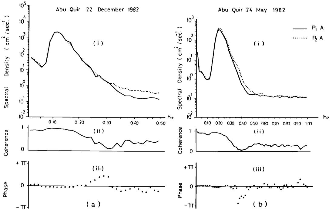
Figure 3. Frequency spectra for two pressure sensors P1A, P2A (i), Coherence (ii), and Phase Difference (iii).
