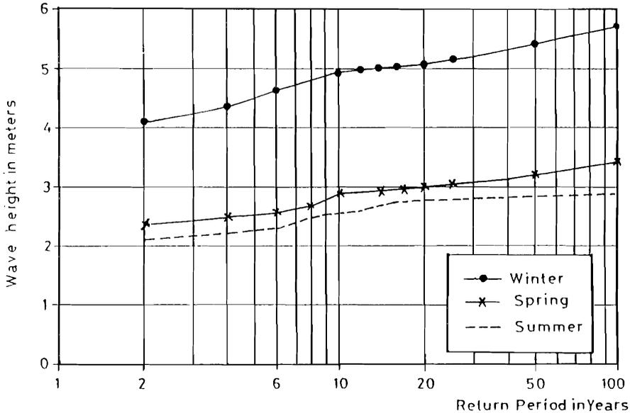
Figure 9. Return periods of storm waves computed from measured at Abu-Quir during the period from 1971 through 1986.
