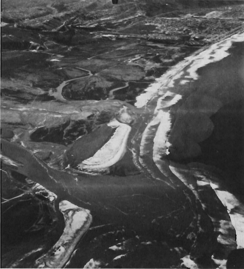
Figure 13. Oblique aerial photograph of the Tijuana River inlet during flooding in 1980. The inlet experienced extreme scouring, and the barrier beach was breached from high stream stormflow discharges.
