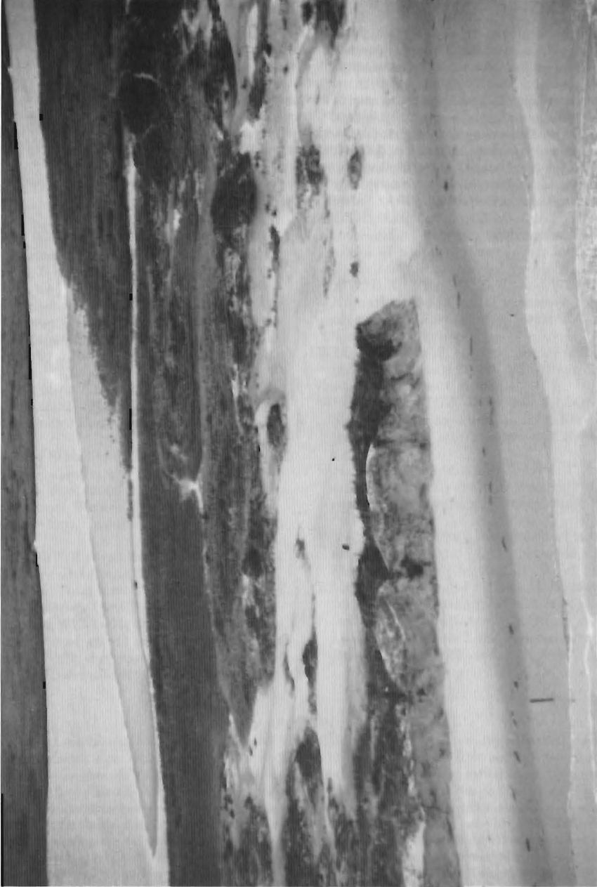
Washover fan on Ocean Isle, North Carolina. Storm surge and waves from Hurricane Hugo eroded and breached this dune field at Ocean Isle, North Carolina, creating a large washover fan. Up to 30 m of dune erosion occurred in this area as a result of the hurricane; narrower dunes were often completely removed or breached. The quantity of sand moved landward as washover is significant: this deposit is up to 1.5 m thick, and covers nearly 500 m 2 . (Photograph: Duke University Program for the Study of Developed Shorelines, Durham, North Carolina. Courtesy of Robert Thieler).
