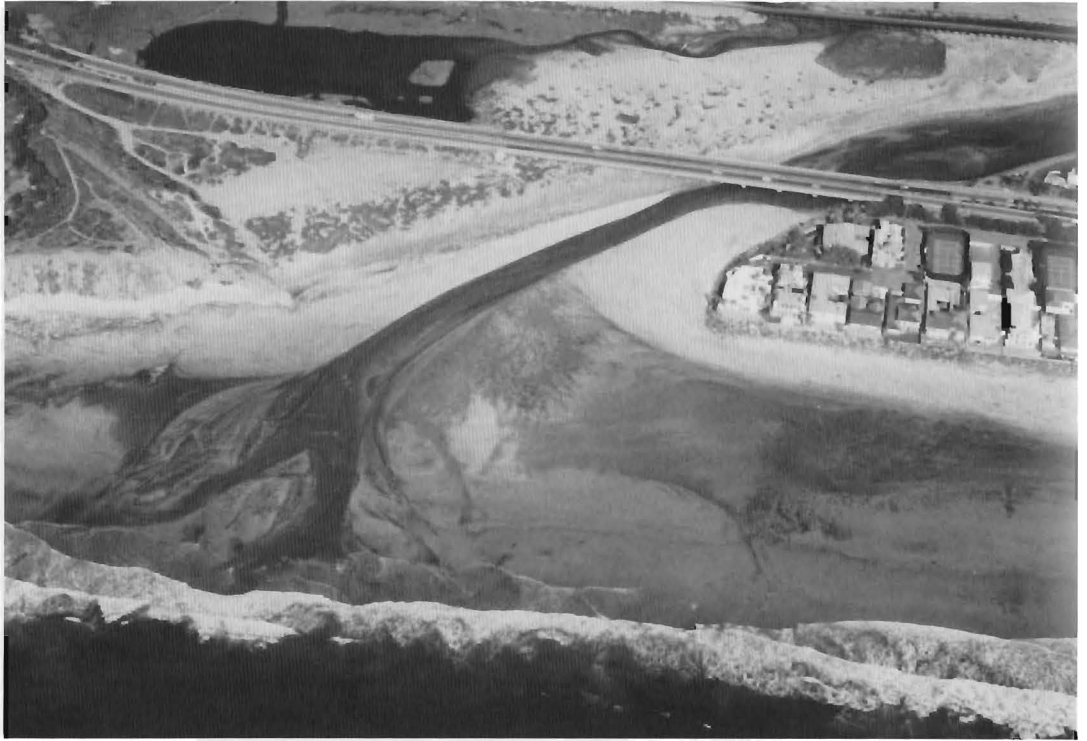
Figure 10. Oblique aerial photograph of the San Dieguito River inlet acquired at low tide on January 27, 1988. The inlet was open and in a linear alignment with the slough. Note that the wave breakpoint was deflected offshore from the inlet as a consequence of delta formation and low spring tide conditions.
