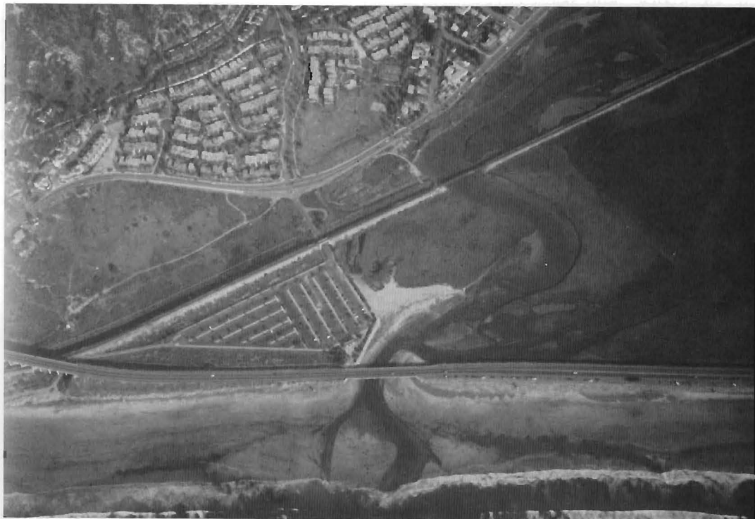
Figure 9. Oblique aerial photograph of Los Penasquitos Lagoon inlet acquired at low tide on January 27, 1988. West is to the bottom of the photograph. The inlet was open during spring tides and stormflow conditions. Note the influence of cobble-size sediment on the form of a braided channel cutting through the delta seaward of the bridge.
