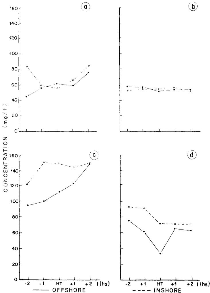
Figure 2. Suspended sediment concentration for the offshore and inshore zones during: (a) survey C1, (b) survey C2, (c) survey C3, (d) survey C4.
