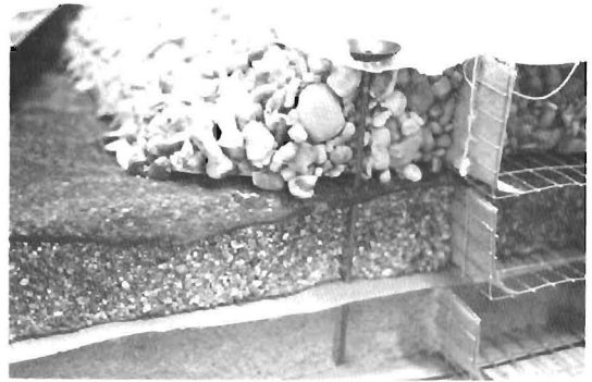
Figure 19. A graded-filter foundation mattress constructed of both natural and synthetic materials offers protection against: (1) scour and currents, (2) piping (seepage erosion) induced by the differential head of water when barrier gates are closed, (3) excess pore water pressures caused by pier-placement loading and (4) liquefaction due to storm waves.
