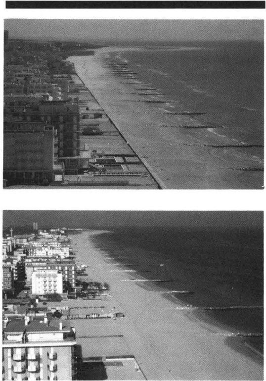
Figure 9. Eastern beach near mouth of the Piave River and effects due to presence of groins, from 1977 (below) to 1987 (top).
