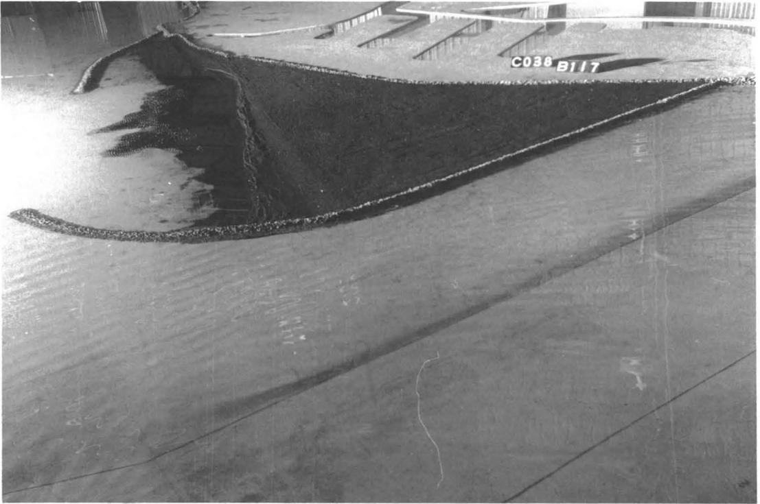
Figure 12. Stable shoreline resulting for optimum improvement plan.
