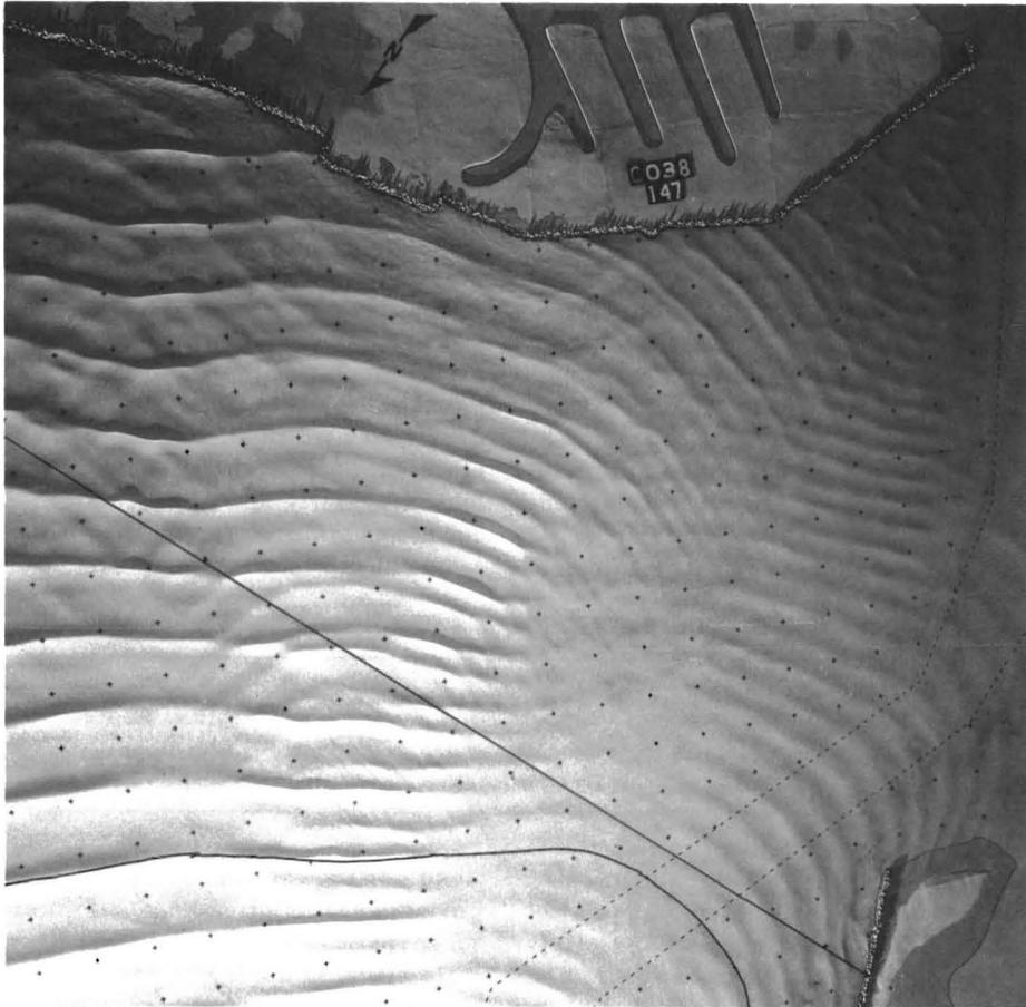
Figure 9. Typical wave patterns approaching Buhne Point in the 1:100-scale model prior to construction of the project.
