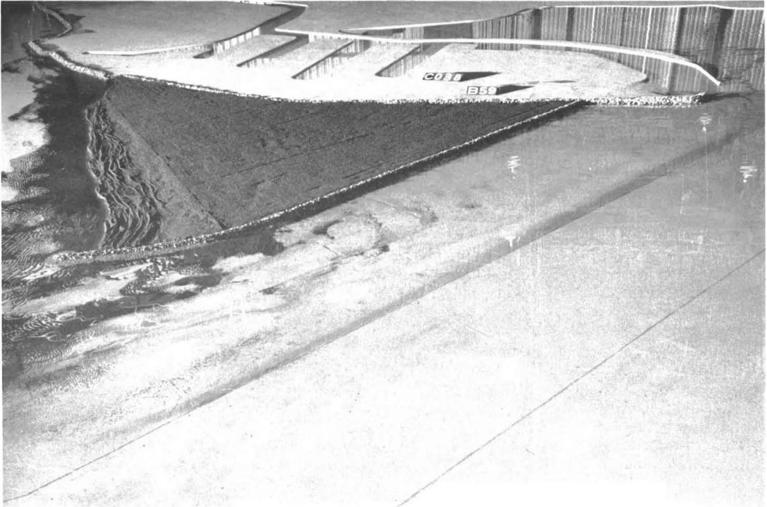
Figure 11. Shoreline configuration showing erosion and accretion for the original test plan.
