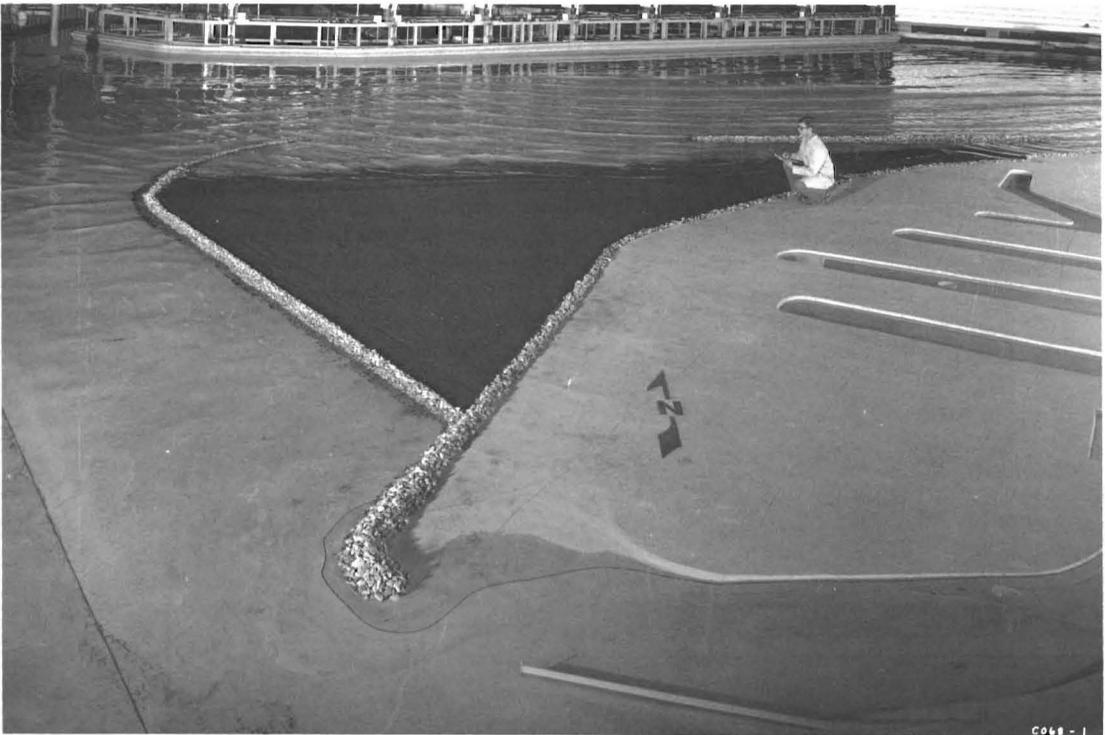
Figure 7 General view of 1:50-scale Buhne Point model with a groin and offshore breakwater plan installed.
