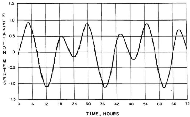
Figure 5. Comparison of computed tidal signal (solid line) versus prototype tide (dashed line) inside Humboldt Bay after calibration.
