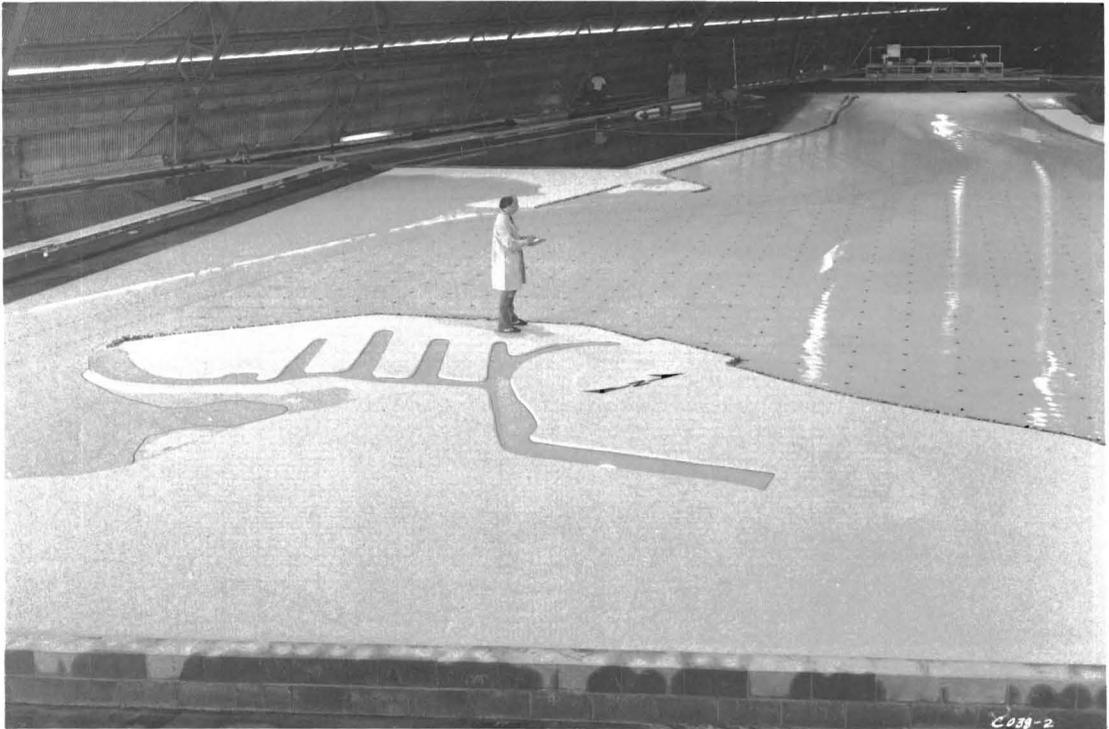
Figure 6. General view of 1:100-scale central Humboldt Bay model prior to modifications.
