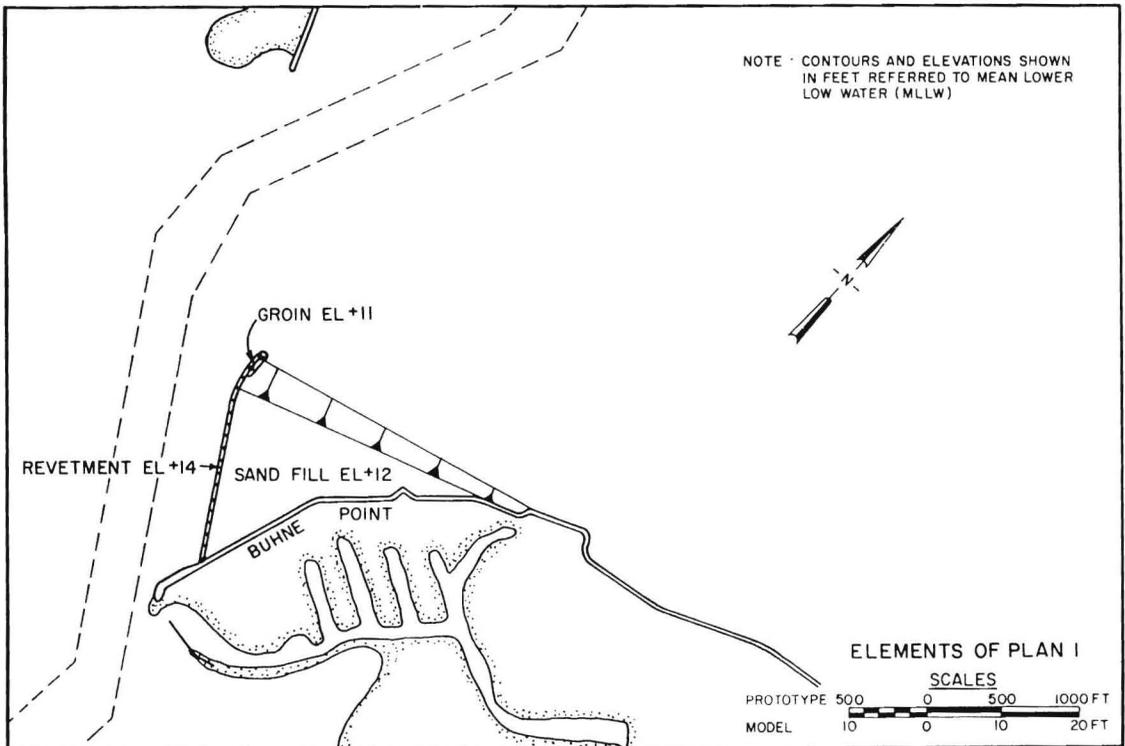
Figure 10. Elements of original improvement plan.
