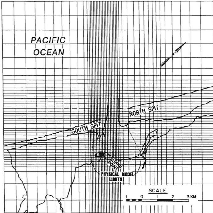
Figure 4. Finite difference grid for the numerical model.
