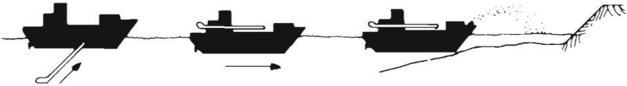
Figure 1(b). Trailing suction hopper dredger pumping through nozzle placed in the bow (CUR, Holland, 1987; see also Bruun, 1988).
