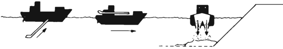
Figure 1(a). Direct dumping in the nearshore zone with hopper dredgers or hopper barges (CUR, Holland, 1987).
