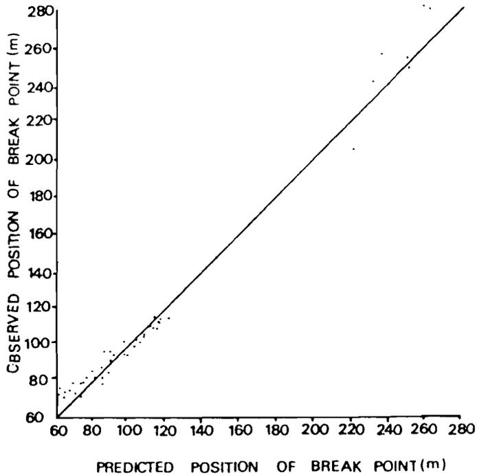
Figure 3. Comparison of the observed breakpoint positions with the predicted positions using McCowan's criteria and breaker parameter value of  $B_o = 0.78$ .
