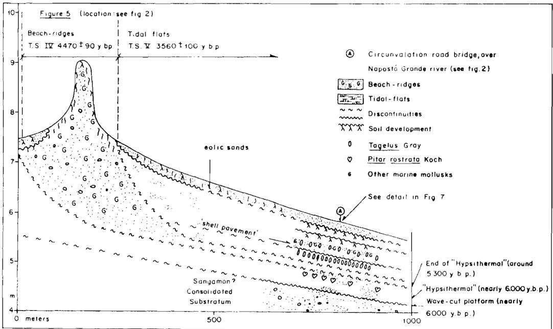
Figure 5. Cross-section over Holocene beach-ridges and tidal flats, middle estuary (E-F in Figure 2).
