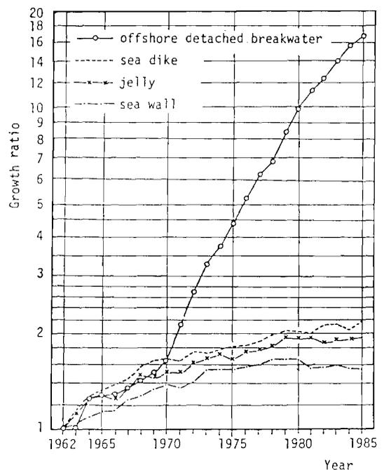
Figure 1. Growth ratio of construction sites for coastal structures.
