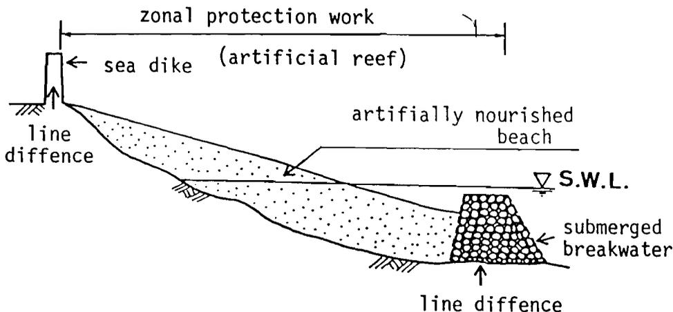
Figure 6. Sketch of a zonal protection system, artificial reef.
