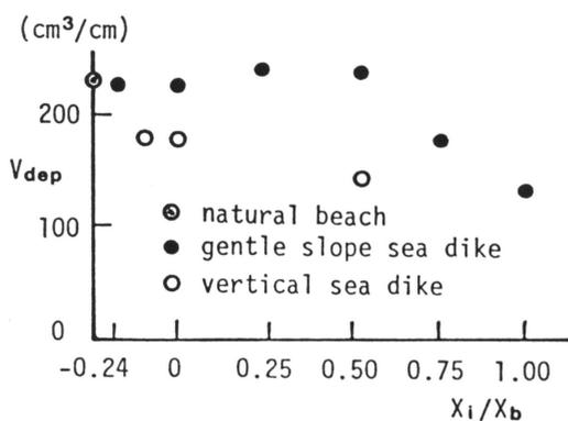
Figure 5. Sand volume deposited in front of sea dikes with different slopes at various locations.
