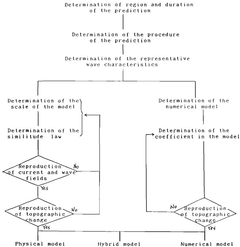
Figure 4. Flow chart for the prediction of beach deformation.
