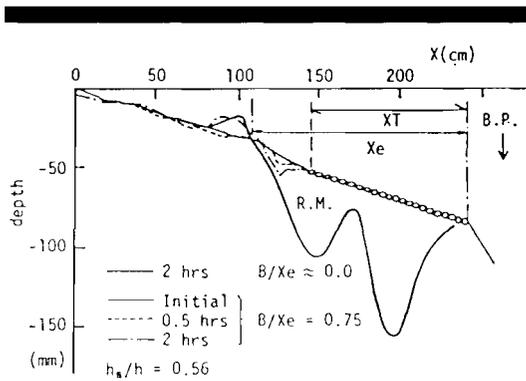
Figure 10. Effect of the width of submerged breakwaters on the deformation of artificial reefs.
