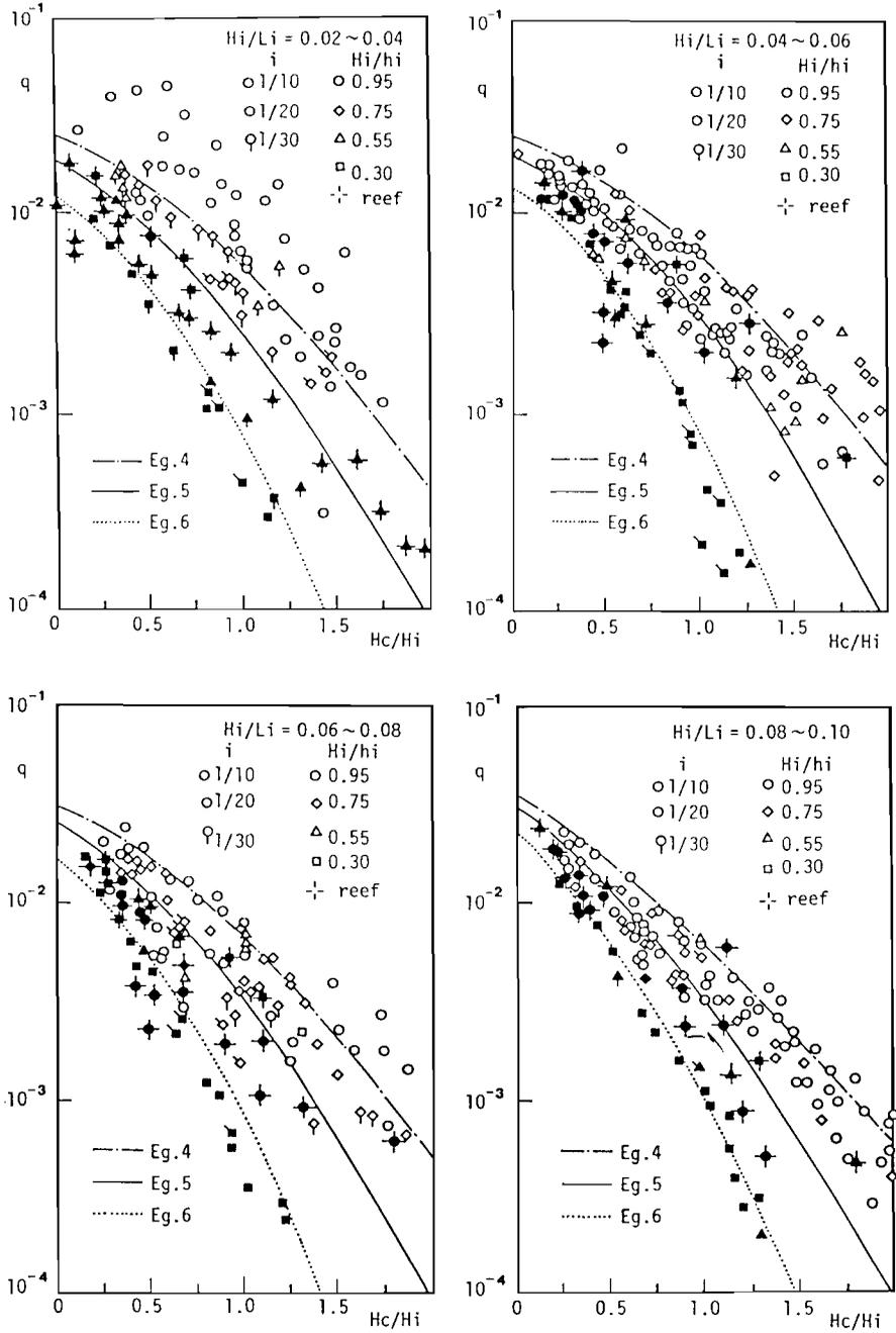
Figure 9. Relation between nondimensional wave overtopping rates and nondimensional crest height of sea dikes.
