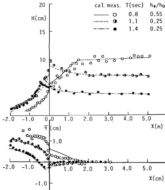
Figure 8. Wave heights and mean water levels on artificial reefs.
