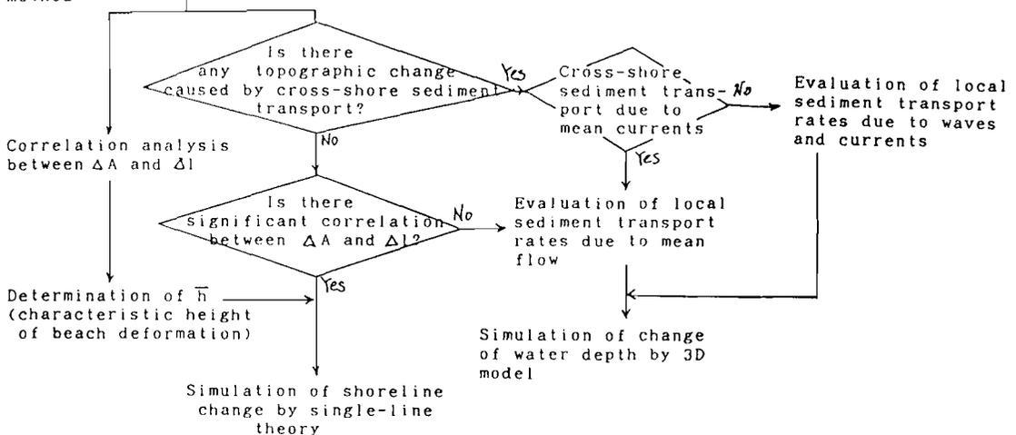
Figure 3. Flow chart for the determination of a beach deformation model for numerical prediction.
