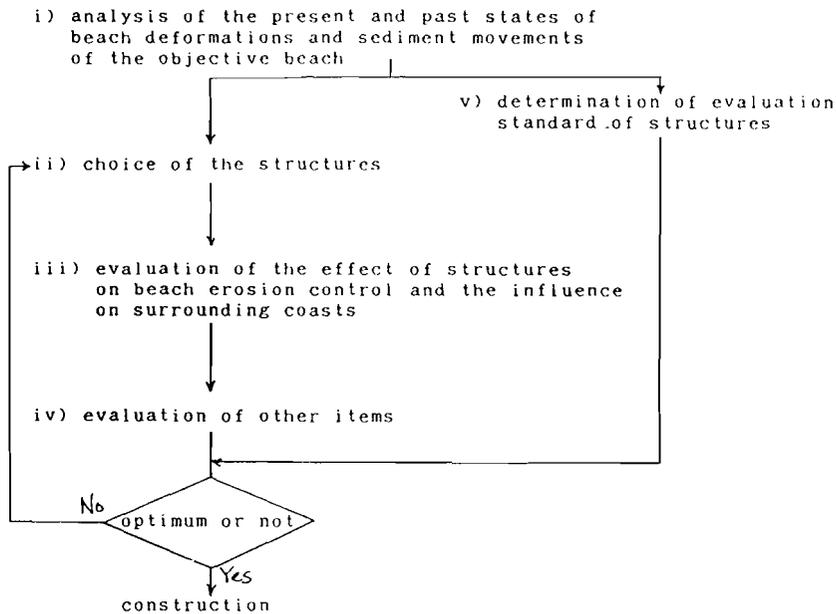
Figure 2. Flow chart for the determination of protection works.
