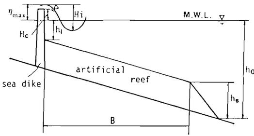
Figure 7. Sketch showing wave overtopping.
