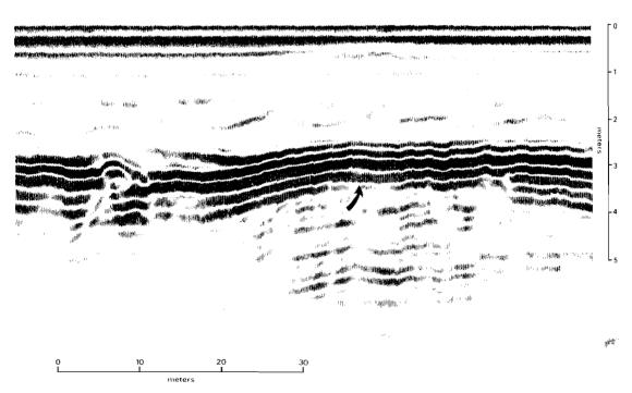
Figure 1. Ground-penetrating radar (GPR) record, indicating shallow peat deposit at 3.5 meters below the surface at Watch Hill on Fire Island, New York. Peaty deposits result in a broken or confused record as compared to the strong, distinct radar signal return from sandy barrier sediments. The chart paper is calibrated in nanoseconds of time, which can be converted to depth according to the travel time for different lithologies as delineated here by vibracoring.
