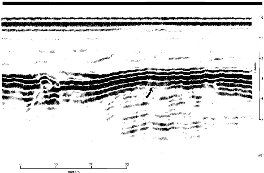
Figure 1. Ground-penetrating radar (GPR) record, indicating shallow peat deposit at 3.5 meters below the surface at Watch Hill on Fire Island, New York. Peaty deposits result in a broken or confused record as compared to the strong, distinct radar signal return from sandy barrier sediments. The chart paper is calibrated in nanoseconds of time, which can be converted to depth according to the travel time for different lithologies as delineated here by vibracoring.
