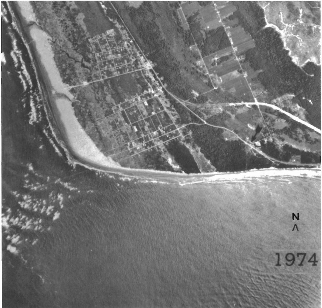
Figure 6. Aerial photograph of Cape Shoalwater taken in 1974. The black arrow indicates the location of the old coast highway threatened by the erosion. The new alignment is under construction to the north.
