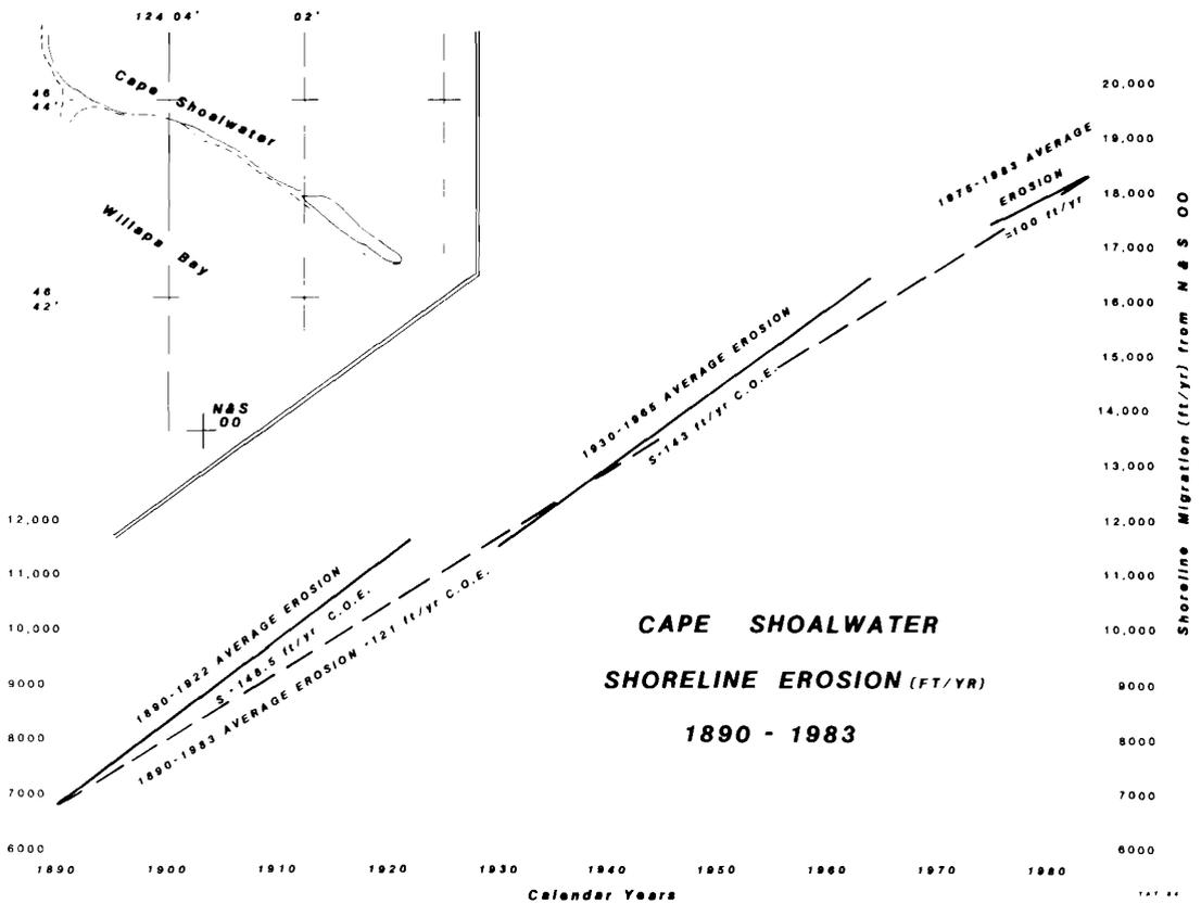
Figure 4. Erosion rates 1890 to 1983. Data 1890 to 1965 by U.S. Army Corps of Engineers, Seattle District. 1975 to 1983 erosion rates calculated by author by measurements from National Ocean Survey charts.
