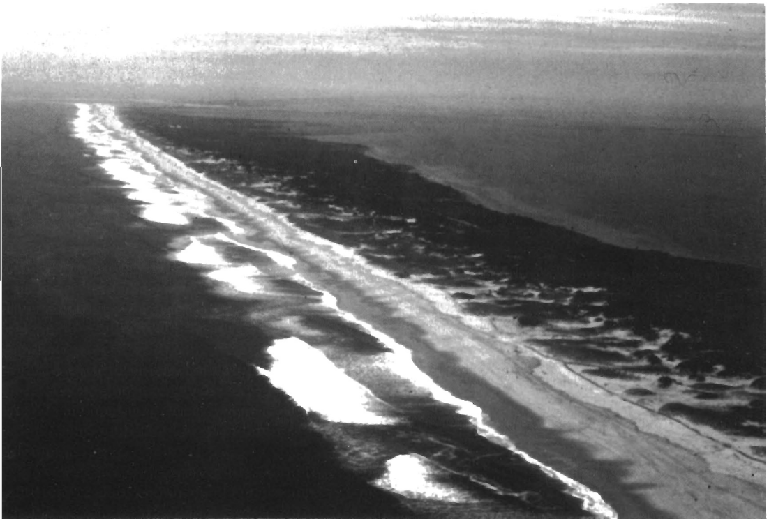
Figure 7B. Air photo looking south along Island Beach reveals circulation cells approximately 500 m wide.
