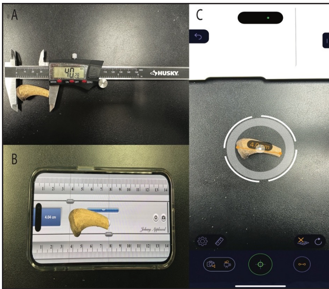
Figure 1: Measuring a bone artifact A) Caliper, B) Ruler app, C) ARuler app
