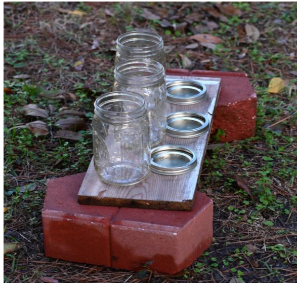
Figure 2. Experimental Setup: Three 32 oz passive deposition jars were elevated 15 cm off the ground using non-plastic materials to collect atmospheric fallout. The setup was unobstructed by trees or buildings, with no contact with heavy foot or vehicle traffic.
