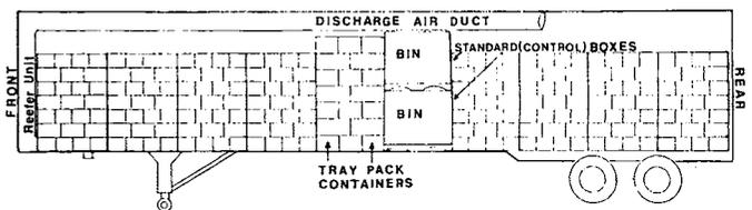
Fig. 4. Diagram showing location of experimental tray-pack containers, bins, and standard (control) boxes in semitrailer van.
