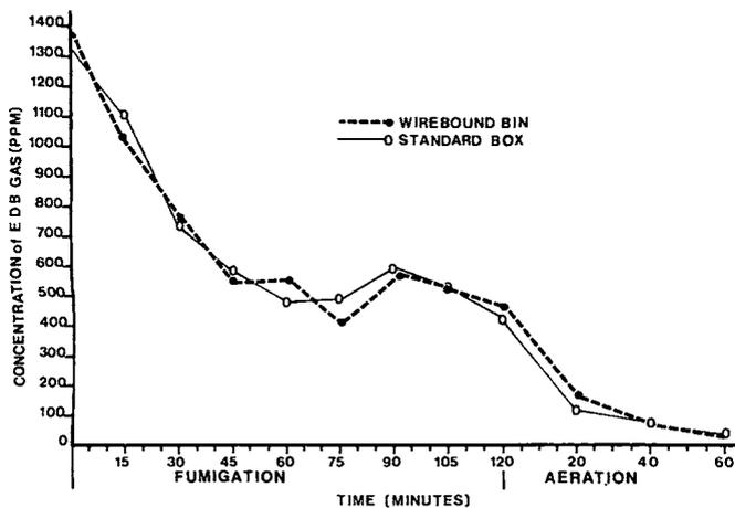
Fig. 6. Concentration of EDB gas (ppm) in semitrailer van in chamber for grapefruit packed in wirebound bins and in standard boxes and placed in a central location of the loads, average of two tests, Florida, 1976-77.
