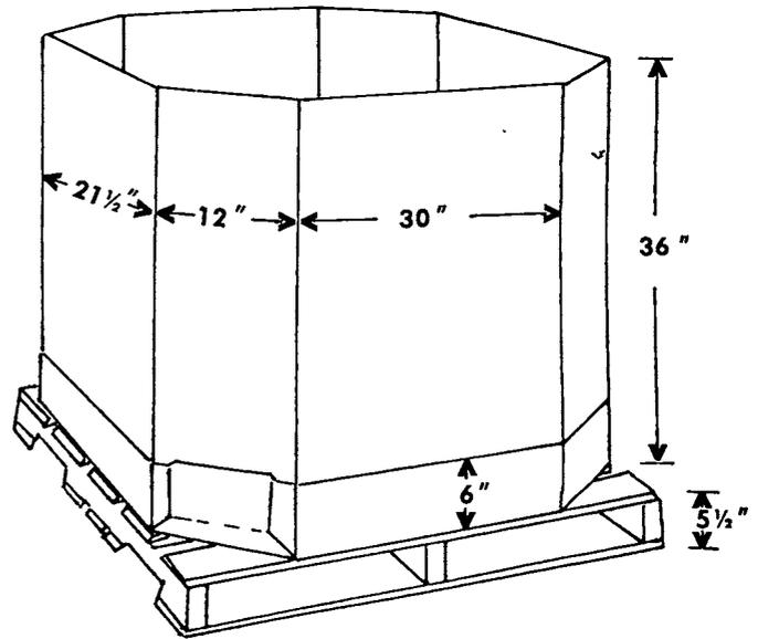
Fig. 3. Diagram illustrating octagonal fiberboard bin. (Note slots in cover cap to provide ventilation through the bin.)
