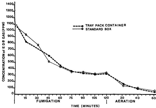
Fig. 5. Concentration of EDB gas (ppm) in a semitrailer van in chamber for grapefruit packed in tray-pack containers and in standard boxes and placed in a central location of the loads, average of four tests, Florida, 1976-77.
