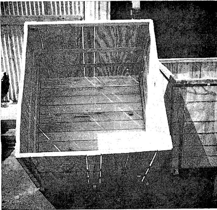
Fig. 2. Wirebound pallet bin on self-contained, wooden pallet base.
