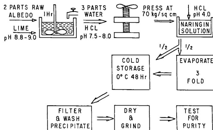
Fig. 1. Naringin extraction using Ca(OH)<sub>2</sub>.
