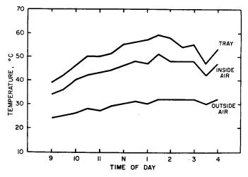
Fig. 2. Temperature profiles in the plywood dryer with no load.
