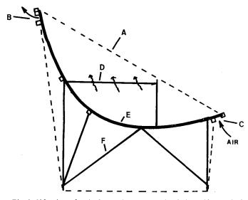
Fig. 1. Side view of strip-frame dryer: A-polyethylene film enclosing dryer; B-slot for exhaust air; C-slot for inlet air; D-food tray; E-parabolic reflector; F-support for the reflector.
