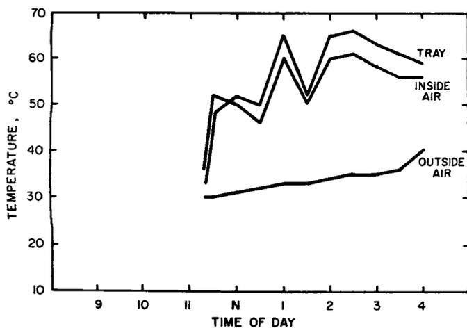
Fig. 3. Temperature profiles in the plywood dryer during peach drying experiment.
