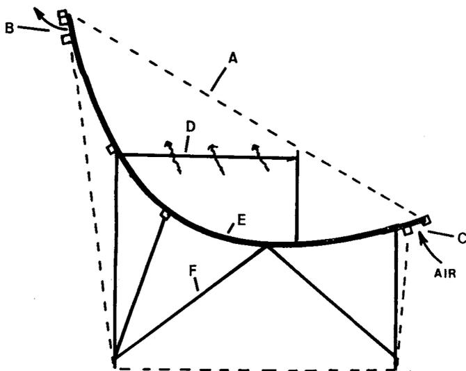
Fig. 1. Side view of strip-frame dryer: A—polyethylene film enclosing dryer; B—slot for exhaust air; C—slot for inlet air; D—food tray; E—parabolic reflector; F—support for the reflector.
