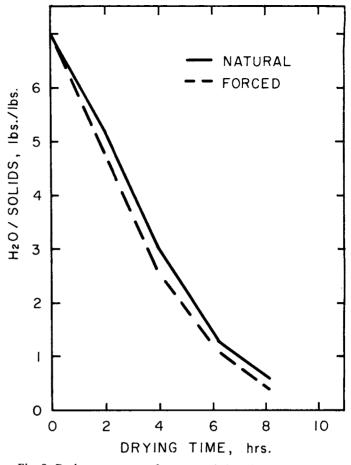
Fig. 2. Drying rate curves for two varieties of mangos each dried in solar dryers with and without forced air circulation.
