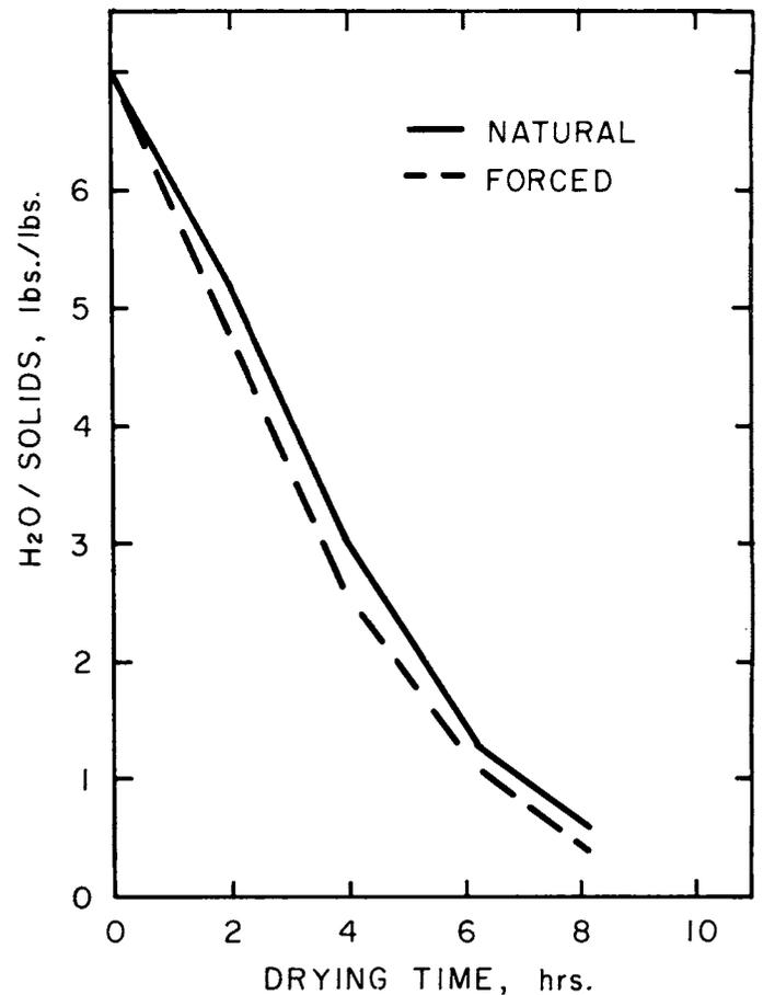
Fig. 2. Drying rate curves for two varieties of mangos each dried in solar dryers with and without forced air circulation.
