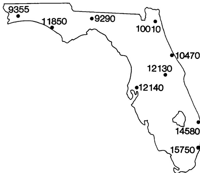
Fig. 2. Simulated yearly consumption of electricity (kw-hr) for air conditioning concrete block control house for each Florida location.
