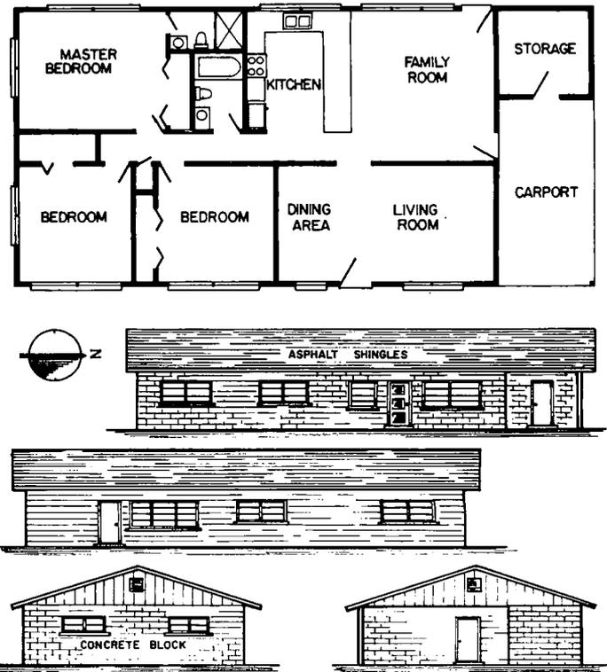
Fig. 1. Floor plan and side views of concrete block control house.
