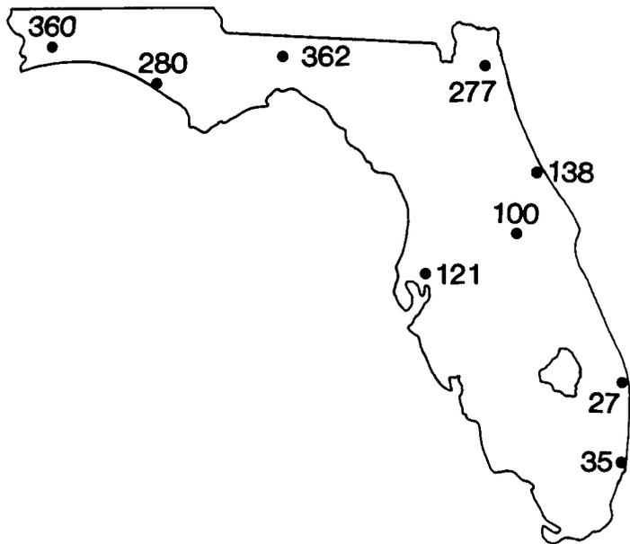
Fig. 3. Simulated yearly consumption of No. 2 residual fuel oil (gallons) for heating the concrete block control house for each Florida location.
